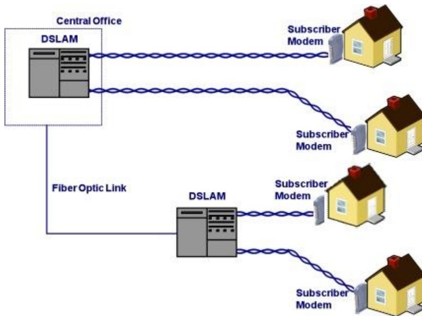
Voice services utilize only a small fraction of the total information carrying capacity of copper connections. In an analogous manner to Ethernet technology, which can transmit a Gigabit (more than one billion bits) per second of data over copper connections or the equivalent of tens of thousands of simultaneous phone conversations, DSL exploits the information carrying capacity of copper lines to deliver broadband services over long distances.
