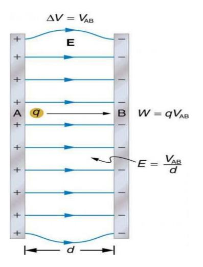
The work done by the electric field in Figure 1 to move a positive charge q from A, the positive plate, higher potential, to B, the negative plate, lower potential, is
