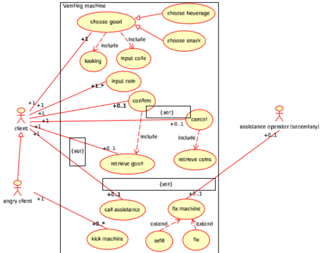
Figure 2.2: The use case diagram of a vending machine.
