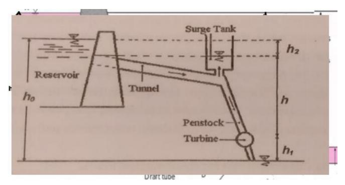
**Reservoir**: Reservoir are built across the rivers to store the water, The water stored on upstream side of dam can be carried by penstocks to the power house.
