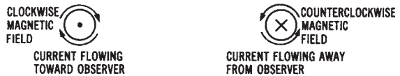
(C) Direction of current flow through conductors determines direction of magnetic field around conductors.
