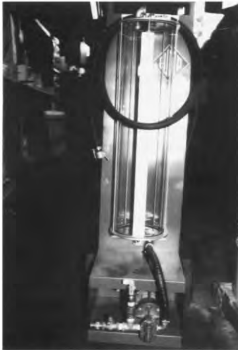
Figure 9. A pneumatically operated portable semi-automatic dispenser. (Courtesy M. A. Drolet, Euclid, Canada.)
