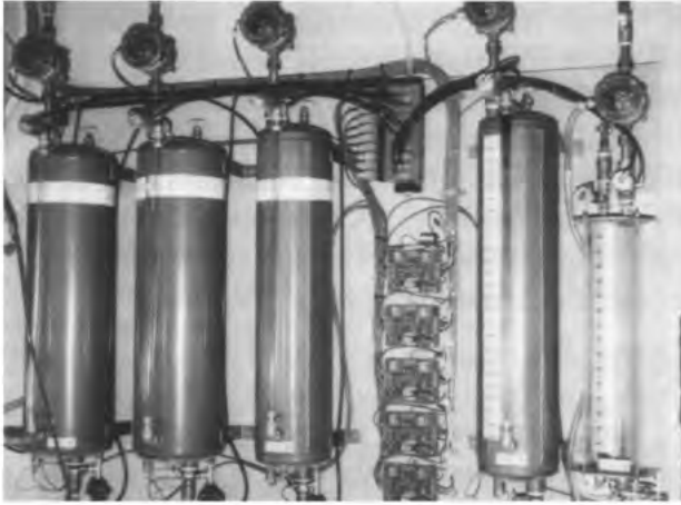
Figure 8. Electrically operated fully automatic dispensers. (Courtesy M. A. Drolet, Euclid, Canada.)
