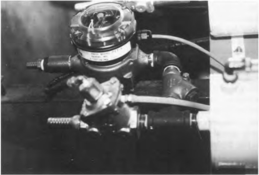
Figure 4. Typical positive displacement flowmeter used for variable admixture dosage. (Courtesy M. A. Drolet, Euclid, Canada.)
