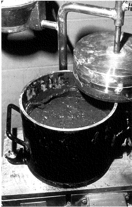
Fig. 3—Determining Vebe time according to ASTM C 1170. Note ring of mortar along side of container.
