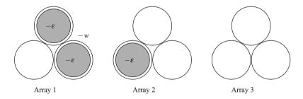
Fig. 5.6 Three triangular arrays of adsorption sites. The *filled circles* represent occupied sites, while the *open circles* are unoccupied. For the configuration shown, we have  $E = -3\varepsilon - w$ .
