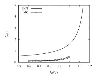
Fig. 7.14 Tolman length versus temperature for the truncated and shifted Lennard–Jones fluid ( $r_c = 2.5\sigma$ ). Monte Carlo (*MC*) simulation employed 8000 particles in a rectangular box (dimension  $20\sigma \times 20\sigma \times 80\sigma$ ) under periodic boundary conditions.
