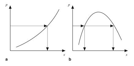
**Fig. C.1** The function p = p(x) can be inverted to give x = x(p) if p = p(x) is monotonic as indicated in **a**. If this is not the case, there may be multiple values of *x* for a given value of *p* as in **b** and the function p = p(x) cannot be inverted.
