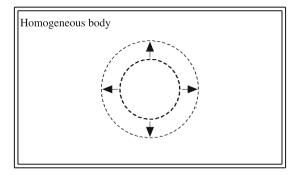
**Fig. 2.12** A system taken inside a homogeneous body is indicated by the *smaller circle*. The *larger circle* represents the system after the infinitesimal change we considered in writing (2.150). Note that the expansion of the system boundary has no effect on the physical state of the matter anywhere in the homogeneous body.
