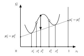
**Fig. 2.21** The common tangent construction to find the mole fractions,  $x_1^c$  and  $x_1^d$ , at phase coexistence. The mixture is unstable between two inflection points (*open circles*) at  $x_1^a$  and  $x_1^b$ .
