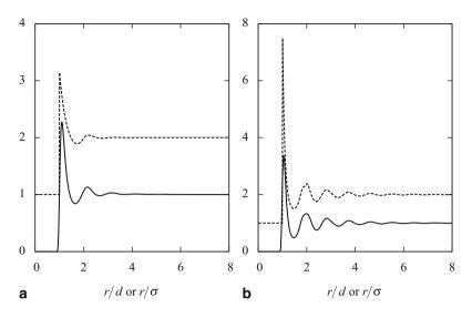
**Fig. 7.5** Comparison of the radial distribution functions of the hard-sphere fluid (*dashed line*) and the truncated and shifted Lennard–Jones fluid (*solid line*) at  $T = \varepsilon/k_B$ . **a**  $nd^3 = n\sigma^3 = 0.5$ . **b**  $nd^3 = n\sigma^3 = 1$ . For clarity, the plots for the hard-sphere fluid are shifted upward by one.
