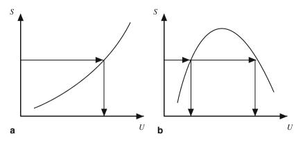
**Fig. 2.2** The function S = S(U), for some fixed values of V,  $N_1, \ldots, N_c$ , can be inverted to give U = U(S) since  $1/T = (\partial S/\partial U)_{V,N} > 0$ , and hence the function is monotonic as indicated in **a**. If 1/T changes its sign as in **b**, there may be multiple values of U for a given value of S and the function S = S(U) cannot be inverted.
