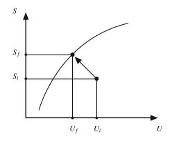
**Fig. 2.10** Graphical illustration of the maximum work principle. The work extracted,  $U_i - U_f$ , is maximum when the arrow connecting the initial state to the final state points horizontally to the left so that  $S_f - S_i = 0$ . In the absence of the external agency,  $U_f = U_i$  and the arrow would point vertically upward as in Fig. 2.8.
