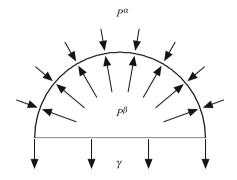
**Fig. 6.9** The surrounding fluid pushes the hemisphere of radius *R* downward with the pressure  $\pi R^2 P^{\alpha}$ , and so does the tension  $\gamma$  with the force  $2\pi R\gamma$ . (From (6.20), we see that  $\gamma$  has the dimension of energy per unit area or force per unit length.) The fluid in the sphere pushes the hemisphere upward with the force  $\pi R^2 P^{\beta}$ . The balance of these forces leads to (6.28).
