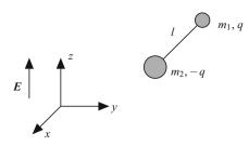
Fig. 3.5 A simple model of a polar molecule.
