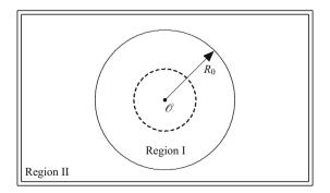
Fig. 6.3 An isolated system containing a metastable vapor phase and a spherical liquid droplet (*dashed line*). The sphere of radius  $R_0$  (*solid line*) separates the isolated system into regions I and II.
