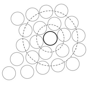
Fig. 7.3 Formation of coordination shells (*gray circles*) around a particle at *r* (*black circle*). Radii of the *dashed circles* are *d* and 2*d*.
