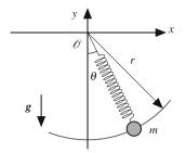
Fig. 1.9 A pendulum suspended by a harmonic spring.
