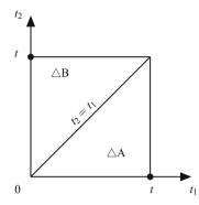
**Fig. 8.1** The integral (8.284) is carried out over the *lower triangle* ( $\triangle A$ ) while (8.285) is over the *upper triangle* ( $\triangle B$ ). Taken together, they cover the square.
