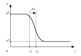
Fig. 6.11 The number density profile n(z) of molecules across a flat interface. Two possible choices are shown for the dividing surface.
