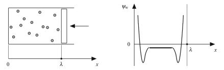
Fig. 3.4 Gas particles confined to a cylinder. Each particle is subject to the external field generated by the walls of the cylinder. The figure on the *right* illustrates the net field  $\psi_w$  produced by the vertical wall on the left and the piston on the right.
