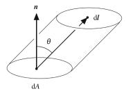
Fig. 2.1 The volume of the column swept out by the surface element dA as it moves by dl is given by  $dl \cdot n dA = dA || dl || \cos \theta$ , in which *n* is the outward unit normal of dA and  $|| dl || \cos \theta$  is the height of the column.
