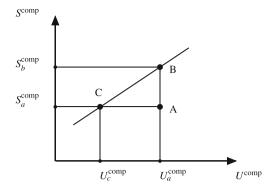
**Fig. 2.14** The entropy change  $\Delta S^{\text{comp}} = S_b^{\text{comp}} - S_a^{\text{comp}}$  for the spontaneous process  $A \rightarrow B$  is related to the energy difference  $W^{\text{rev}} = U_c^{\text{comp}} - U_a^{\text{comp}}$  by (2.179).
