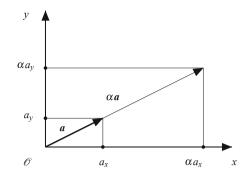
Fig. A.2 Components of *a* and multiplication of a vector *a* by a number  $\alpha$ .
