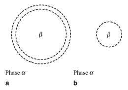
Fig. 6.2 A droplet ( $\beta$ ) in equilibrium with a supersaturated vapor  $\alpha$ . At a lower degree of supersaturation, the droplet attains bulk-like properties near its center, a situation we indicate with a pair of *dashed circles* in **a**. At a higher degree of supersaturation, however, it becomes inhomogeneous even at its center as indicated by a *single dashed circle* in **b**.
