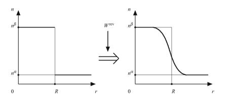
**Fig. 6.10** Introduction of an interface into the reference system by means of a reversible work source. The number density of molecules is denoted by *n* with a *superscript* indicating its values in the bulk reference phases.
