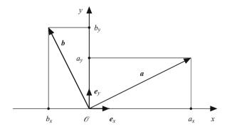
Fig. A.1 Components of two-dimensional vectors *a* and *b*.
