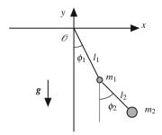
Fig. 1.8 A coplanar double pendulum oscillating in the xy-plane. Both  $l_1$  and  $l_2$  are constant.
