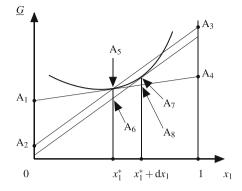
Fig. 2.19 Graphical derivation of the Gibbs–Duhem relation for a constant (T, P) process in a binary mixture.
