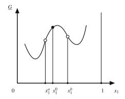
**Fig. 2.18** <u>*G*</u> versus  $x_1$  plot at constant (T, P) showing two inflection points indicated by the *open circles*.
