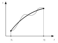
**Fig. 1.6** The actual path z(t) followed by the mechanical system (*thick curve*) and a varied path  $z'(t) = z(t) + \delta z(t)$  (*thin wavy curve*). Note that  $\delta z = 0$  at  $t_1$  and  $t_2$ .
