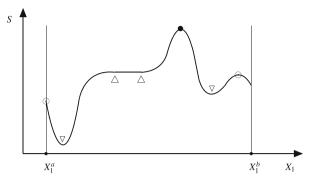
**Fig. 2.5** Various possible states of equilibrium when  $X_1$  is confined to the interval  $[X_1^a, X_1^b]$ . The system is in stable (•), metastable ( $\odot$ ), unstable ( $\bigtriangledown$ ), and neutral equilibrium (between the two  $\triangle$ ).
