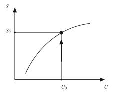
Fig. 2.8 Projection onto the US-plane of the locus of the maximum entropy as a function of U. The vertical arrow at  $U_0$  indicates the trajectory of the system during evolution toward equilibrium as observed in the US-plane. The *filled circle* indicates the state of equilibrium after the partition became diathermal.
