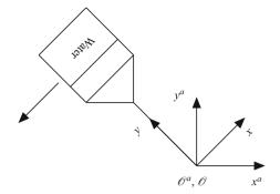
Fig. 3.7 A rotating bucket of water as observed from the inertial frame  $\mathcal{O}^a$  and the frame  $\mathcal{O}$  that rotates with the bucket.
