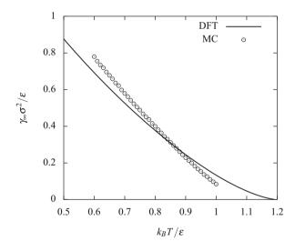
Fig. 7.13 Surface tension versus temperature for the truncated and shifted Lennard–Jones fluid ( $r_c = 2.5\sigma$ ). Monte Carlo (*MC*) simulation employed 8000 particles in a rectangular box (dimension  $20\sigma \times 20\sigma \times 80\sigma$ ) under periodic boundary conditions.
