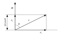
**Fig. 3.8** Decomposition of *r* into  $r_{\perp}$  and  $r_{\parallel}$ .
