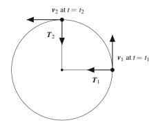
Fig. 1.5 In the case of a particle moving on a circle at a constant speed, the velocity v changes its direction without changing its length. A force is still needed to change the direction of v and is supplied, for example, by the tension T in a string to which the particle is attached. The work W done on the particle by T, however, is zero.
