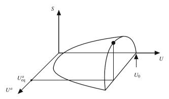
**Fig. 2.7** Graphical representation of *S* of the composite system considered in Sect. 2.8.2. In drawing this graph, all the variables occurring in (2.80), except for *U* and  $U^a$ , are fixed. The equilibrium value of  $U^a$ , which we denote here by  $U^a_{eq}$  is determined so that *S* takes the maximum possible value consistent with the given value,  $U_0$ , of the internal energy of the composite system. The equilibrium state is then indicated by the *filled circle*.
