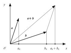
Fig. A.3 Addition of two vectors *a* and *b*.
