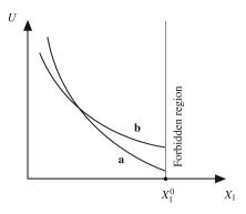
**Fig. 2.9** The function  $U = U(X_1)$ . Suppose that  $X_1$  cannot exceed  $X_1^0$  and the slope of U at  $X_1 = X_1^0$  is negative initially as indicated by curve **a**. As illustrated by curve **b**, the slope remains negative even after an infinitesimal change is made to *S*. Then,  $X_1 = X_1^0$  at equilibrium both before and after the change. So,  $\Delta X_1 = 0$ .
