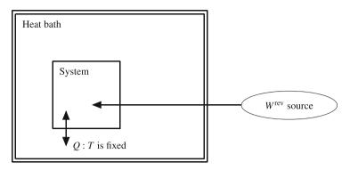
Fig. 2.13 The system of interest in contact with a heat bath. The reversible work source is connected only to the system and not to the heat bath.
