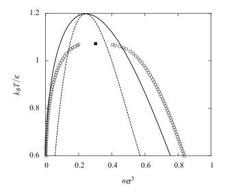
Fig. 7.11 Phase diagram of the truncated and shifted Lennard–Jones fluid ( $r_c = 2.5\sigma$ ). The binodal (*solid line*) and the spinodal (*dashed line*) lines, both from the density functional theory. The coexisting densities ( $\odot$ ) and the critical point (**n**), both from Gibbs ensemble simulation involving the total of 1000 particles.
