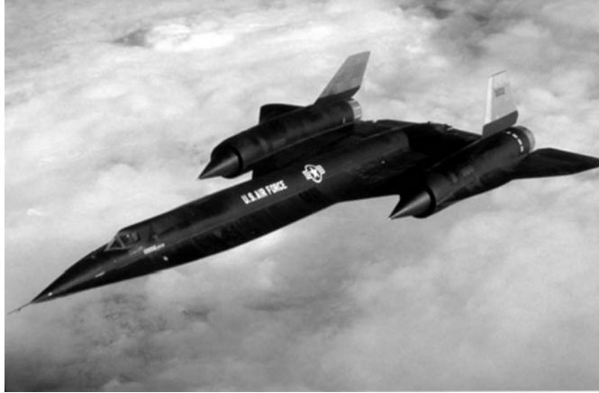
(above) The A-12/OXCART aircraft was developed by Lockheed for the CIA as a successor to the U-2. The plane could fly at over 2,100 miles per hour and at an altitude of over 90,000 feet. The A-12 had a brief operational life, beginning in May 1967 and ending in June 1968, when it was retired in favor of the Air Force's A-12 derivative—the SR-71. CREDIT: Lockheed
