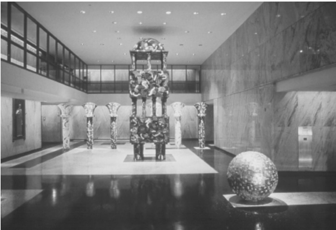
Figure 13.3 Matching luminaire apertures of the same dimension and finish.
