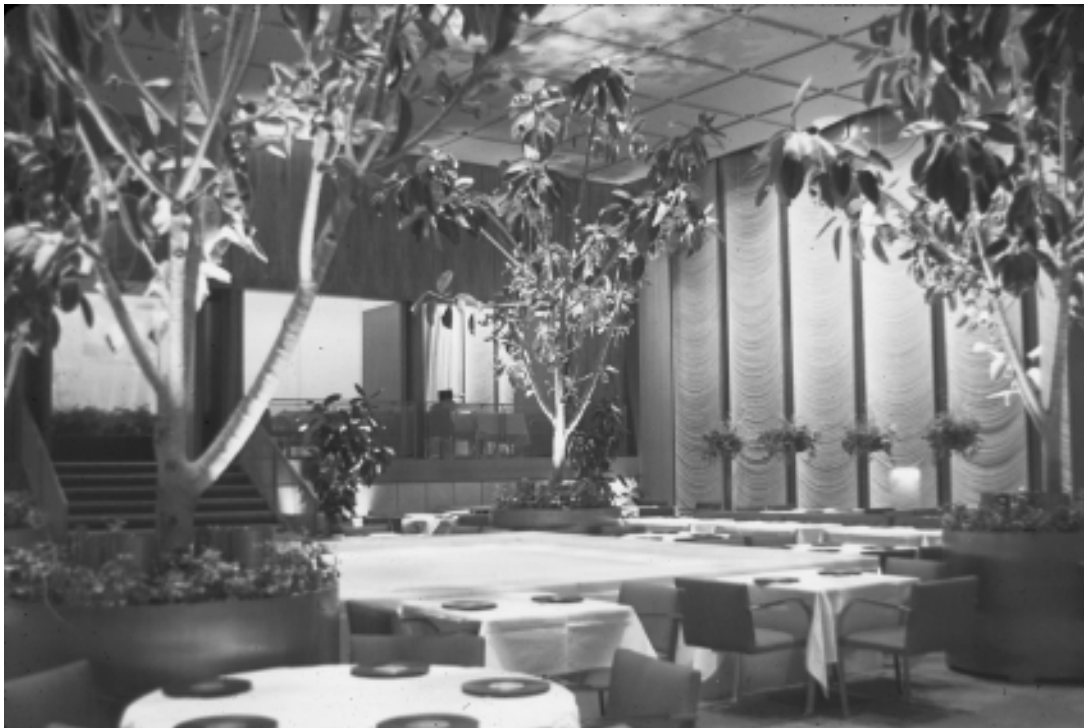
Figure 13.35 When the lighting system illuminates both horizontal and vertical surfaces, the brightness is balanced.
