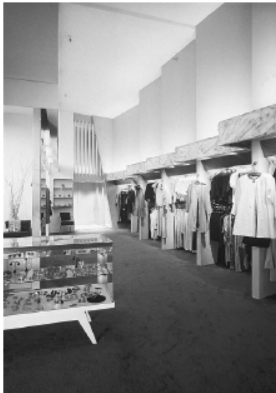
Figure 3.8 An example of concentrated upward distribution with the light source placed farther from the illuminated surface.
