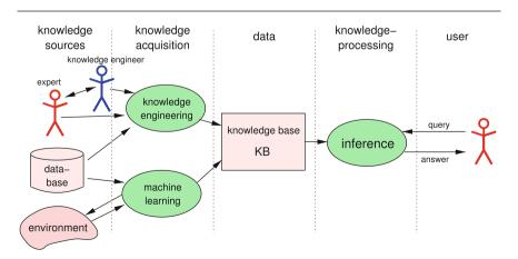
Fig. 1.7 Structure of a classic knowledge-processing system
