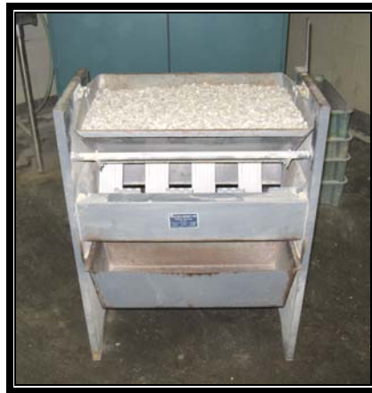
Figure 6 Reducing Sample to Test Size
