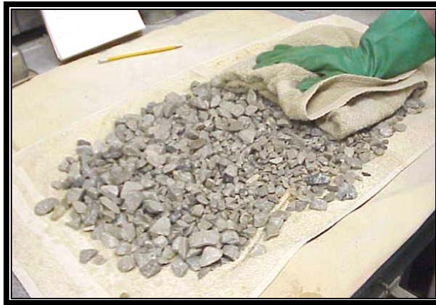
Figure 8 Removing Excess Water
