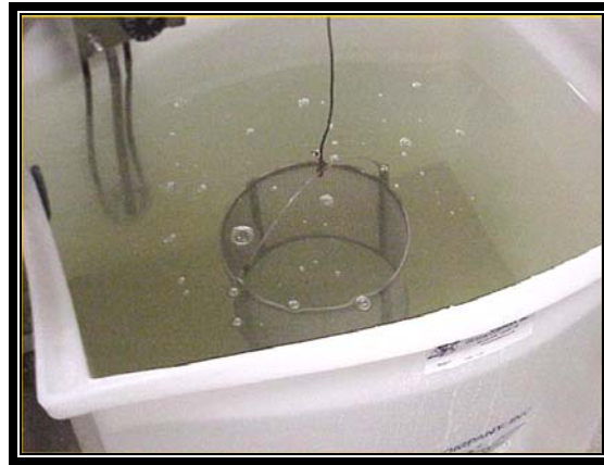
Figure 1 Coarse Aggregate Gravity Apparatus
