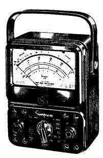
Figure 6-8 Meter with mirrored scale.
