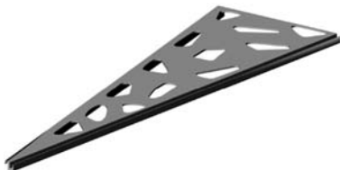
Fig. 7.64 Triangular UHPC element for cladding to Jean Bouin Stadium, Paris [172]
