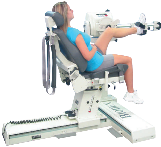
Figure 20.11 Use of a commercially available dynamometer to measure force during a knee extension.
