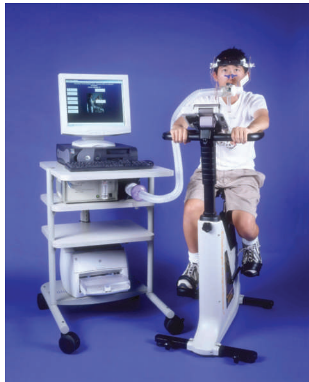
Figure 1.4 The TrueOne metabolic measurement system utilizes electronic flow sensors, gas analyzers, and computer technology. These devices are used to measure oxygen uptake and carbon dioxide production at rest and during exercise.
