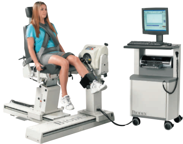
Figure 20.13 Use of a commercially available computer-assisted isokinetic dynamometer to measure strength during a knee extension.
