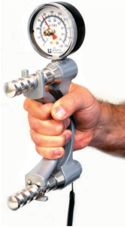
Figure 20.12 Use of the typical hand-grip dynamometer. Photo Courtesy of Lafayette Instrument Company
