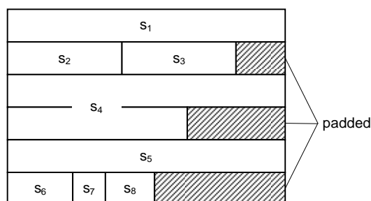
Fig. 1.8. Representation of a packed record
