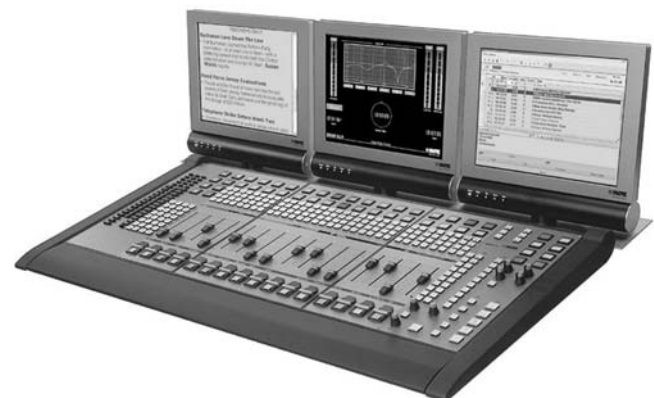
FIGURE 3.5 Digital consoles also incorporate LCD panels. (Image courtesy of Klotz Digital America, Inc.)
