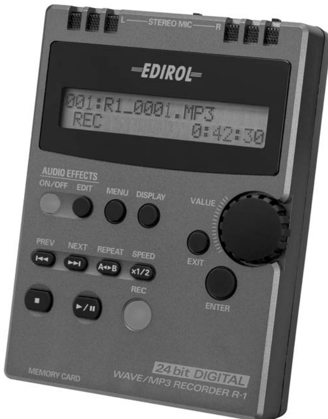
FIGURE 5.12 Some compact flash recorders are designed to be held in your hand with all functional controls at your fingertips. (Image courtesy of Edirol Corporation.)
