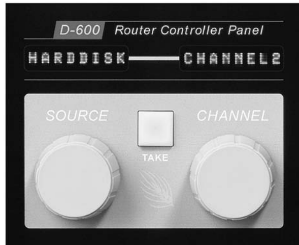
FIGURE 3.7 On most digital audio consoles, any available audio source can be assigned to any one of the console's input channels. (Image courtesy of Wheatstone Corporation.)
