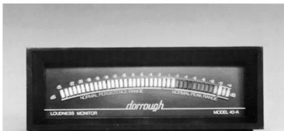
FIGURE 3.11 VU meters with fluorescent or liquid crystal displays can indicate volume changes more quickly and accurately than electromechanical meters. (Image courtesy of Dorrough Electronics.)
