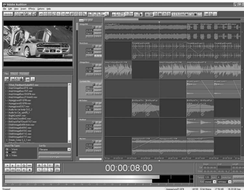
FIGURE 6.3 Most digital audio editing software also incorporates a virtual multi-track recorder. (Adobe product screen shot reprinted with permission from Adobe Systems Incorporated.)
