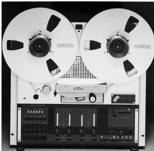
FIGURE 6.6 No longer available, one of the first multi-track recorders used in the radio production studio was a 4-track reel-to-reel recorder. (Image courtesy of Studer Revox America, Inc.)
