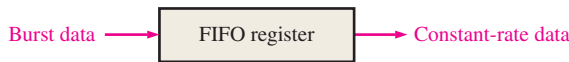
(d) Data in bursts can be stored and reformatted into a constant-rate output.
