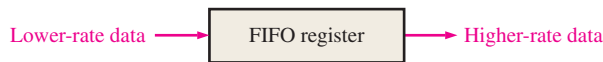
(b) Data input at a slow keyboard rate can be stored and then transferred at a higher rate for processing.
