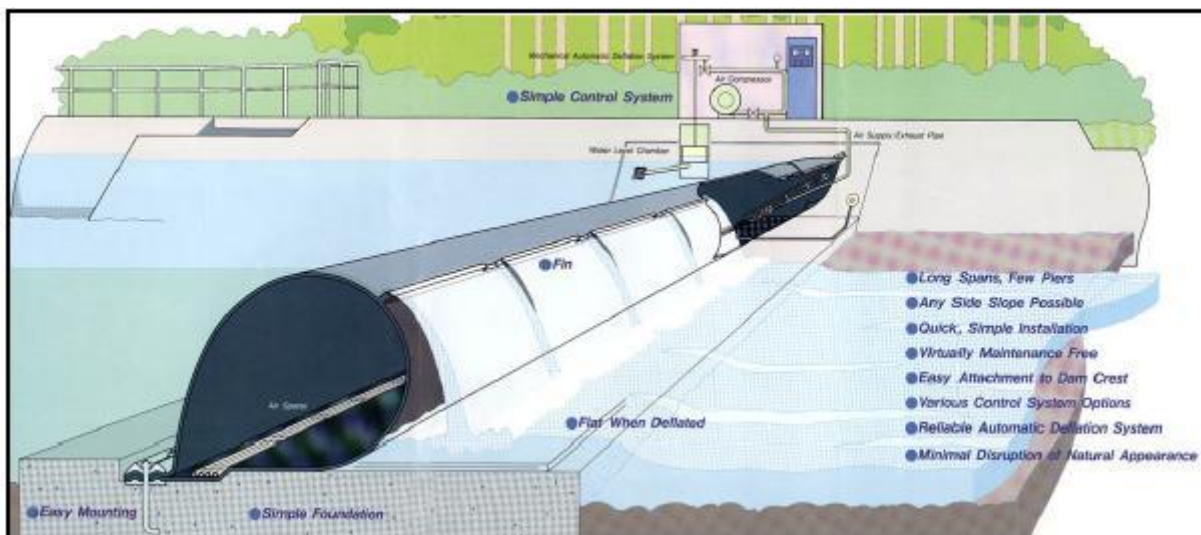
Fig. 2.17 – Schematic view of a Rubber Dam – Courtesy of Bridgestone [3]
