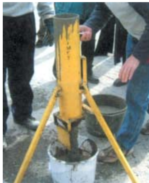
Concrete flowing through Orimet device
