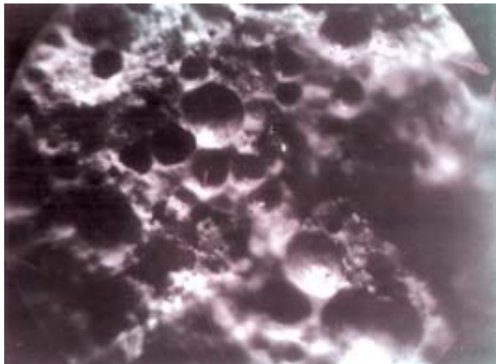
Photograph (25 times magnification) showing the presence of air-entrainment in hardened concrete, generated by Ritha powder as air-entraining admixture. (source M.E. Dissertation work of M.S. Shetty —1964)
