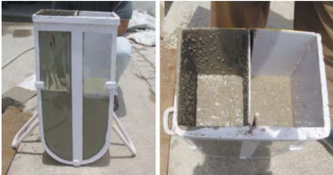
Concrete passing through U-Box Courtesy : Hindustan Construction Company
