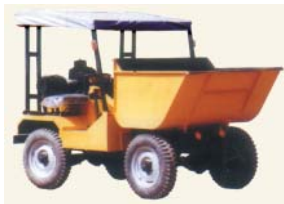
Tough Rider for transporting concrete.
