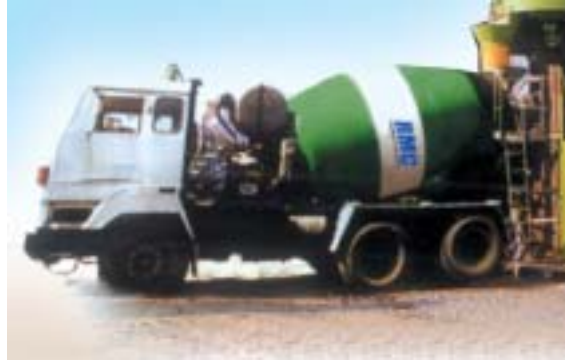
Transit Mixer, a popular method of transporting concrete over a long distance.
