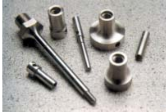
Needle with different bearing area
