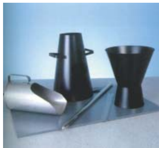
Slump Test Apparatus
