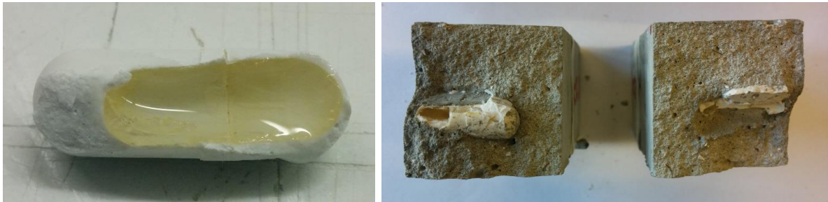
Figure 1 (left) a cross section from a gelatin-IPC capsule containing healing agent (right) a gelatin-IPC specimen embedded in a mortar beam which was then broken by three-point-bending.
