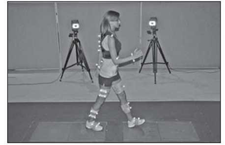
Reflective joint markers can be tracked by a camera for automatic digitizing of the movement.
