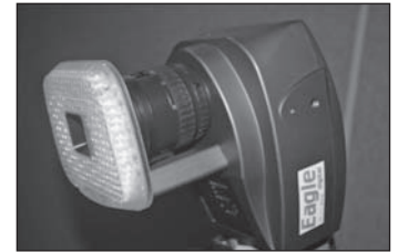
A digital camera with infrared light ring is used for tracking reflective markers on a subject.
