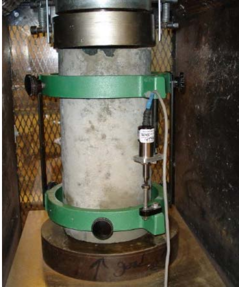
Figure 3-7. Extensometer attached to specimen
