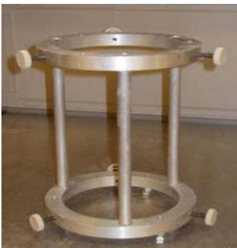
Figure 3-8. Gauge Positioning Guide
