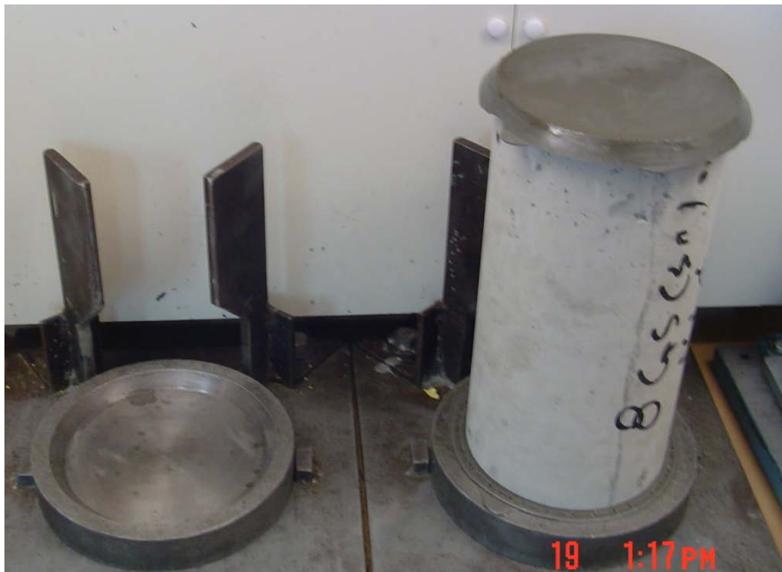
Figure 4-3. Capping procedure for specimen to be tested in creep frame
