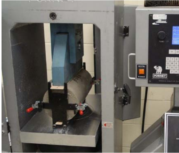
Figure 3-6. Specimen being tested for splitting tensile strength
