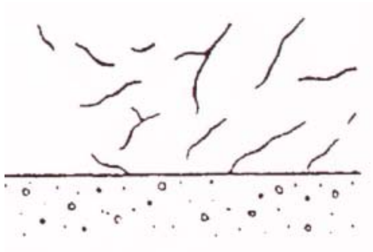
FIG. 2.13. Cracks due to abnormal set of cement.
