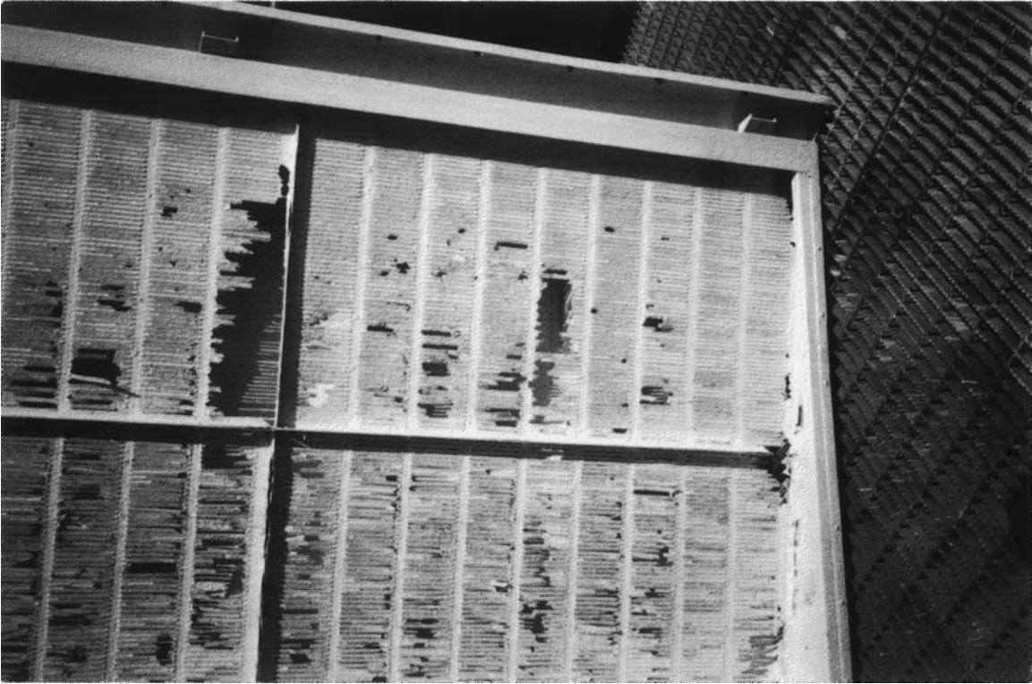
FIG. A-56 A corroded inertia filter. (Source: Altair Filters International Limited.)
