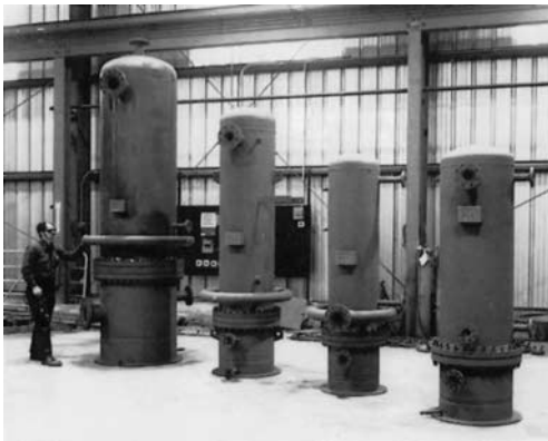
FIG. V-17 Four typical vertical vaporizers for large Mideastern refiner. Note the inlet belts on three of the vaporizers, often used to improve shell side distribution for improved boiling and excessive tube impingement. (Source: Armstrong Engineering Associates.)
