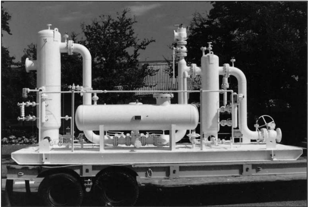
FIG. F-32 System installed in Saudi Arabia includes one vertical dry scrubber followed by two pressure regulating valves and a line separator. A condensate drain tank is mounted alongside. (Source: Peerless.)
