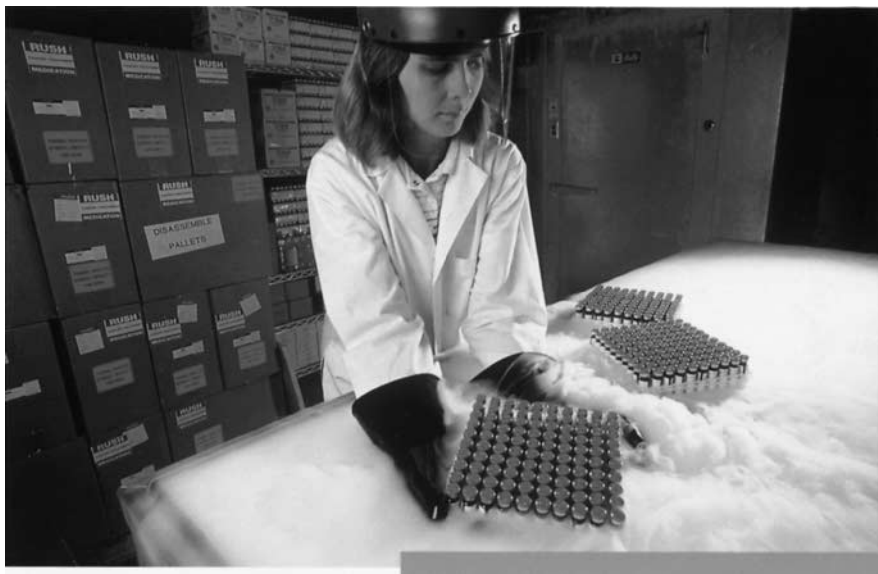
FIG. D-4 Suitable clothing for operator handling. (Source: ARCO Chemical.)
