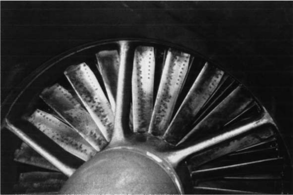
FIG. A-42 A fouled compressor. (Source: Altair Filters International Limited.)
