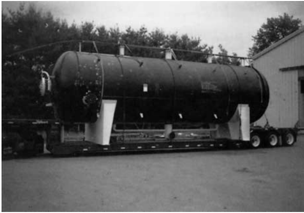
FIG. V-1 Very large low-temperature vaporizer/superheater, steam heated. Unit size 132 in (3353 mm) in diameter by 42 ft (13 cm) long. Duty to boil and superheat very low-temperature organic liquid. (Source: Armstrong Engineering Associates.)
