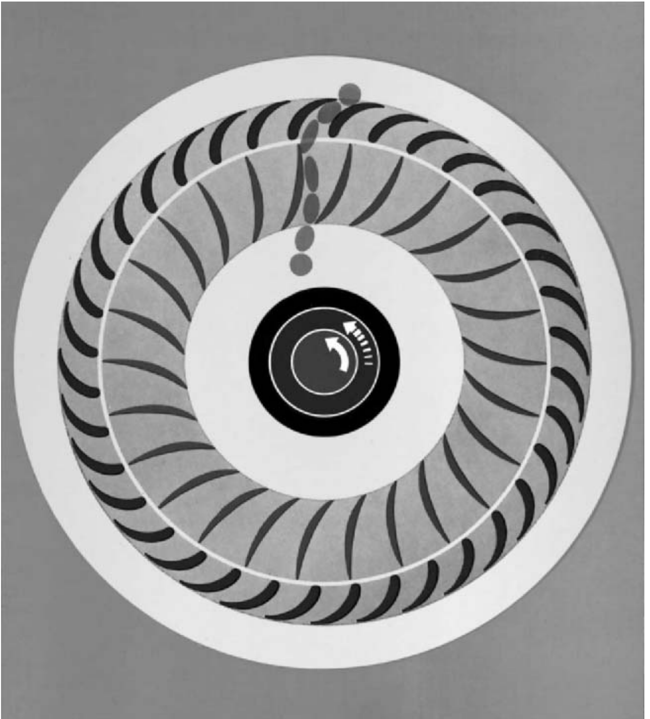
FIG. P-74 Hydrodynamic power transmission (converter). (Source: J. M. Voith GmbH.)
