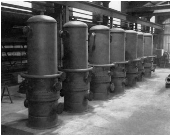
FIG. V-5 Seven large hydrocarbon fluid vaporizers for chemical plant in Middle East. Unit size 36 in (914 mm) in diameter, overall height 135 in (3430 mm). (Source: Armstrong Engineering Associates.)
