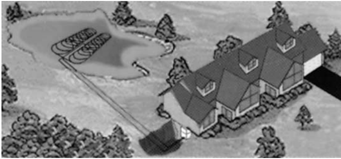
FIG. H-1 Pond and lake loops. (Source: Enertran.)
