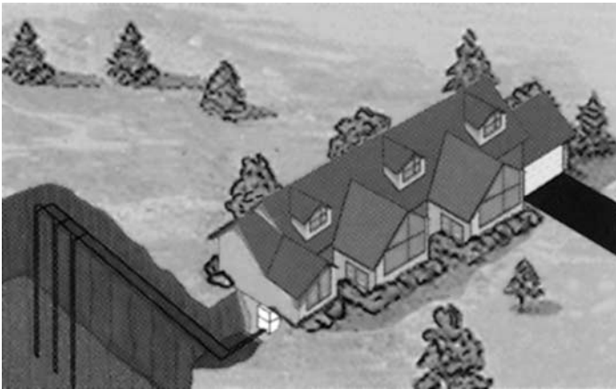
FIG. H-4 Vertical loops. (Source: Enertran.)
