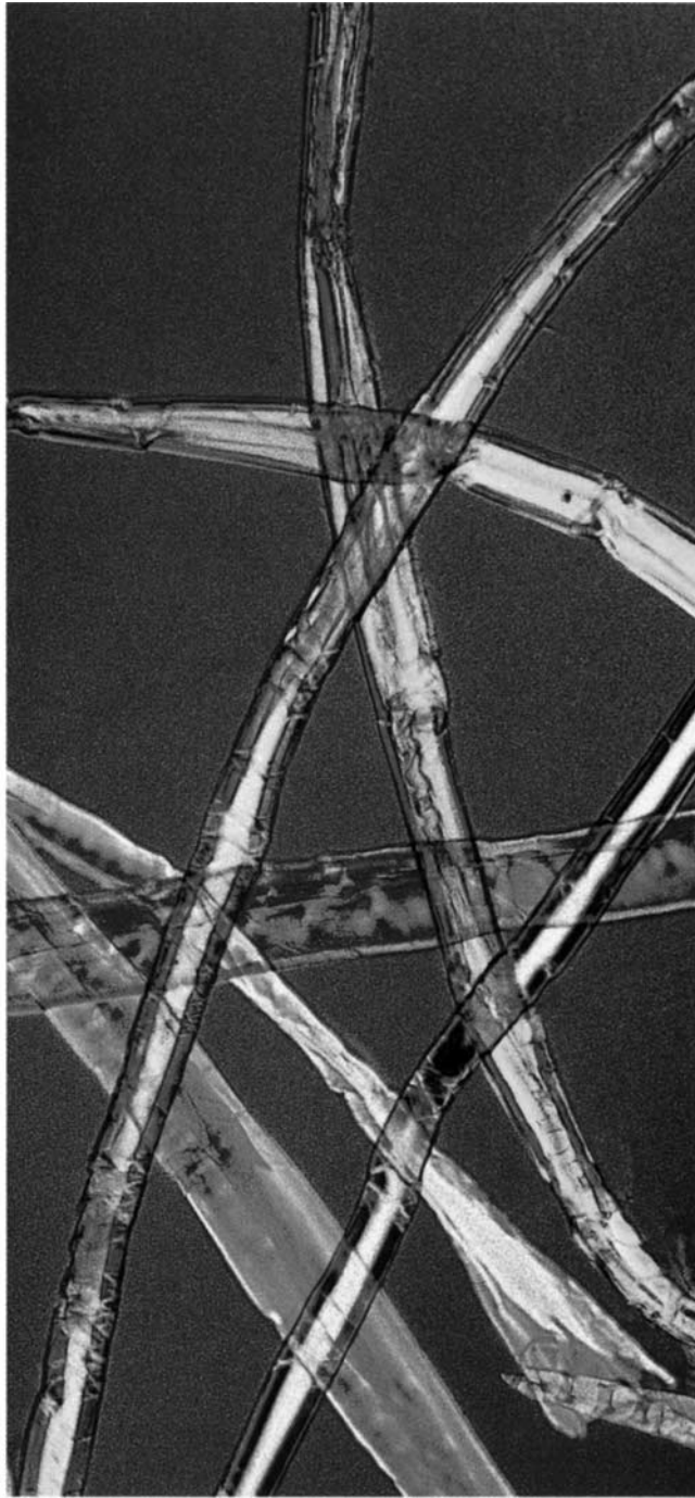
FIG. E-42 Long, strong fibers are a prerequisite for resource-efficient manufacture of strong packaging. The photo shows spruce fibers at a magnification of 100 times. (Source: AssiDomän.)
