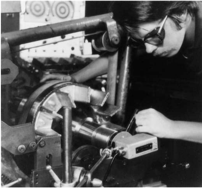
FIG. E-17 Complete rotor assembly is dynamically balanced. (Source: Reliance Electric.)
