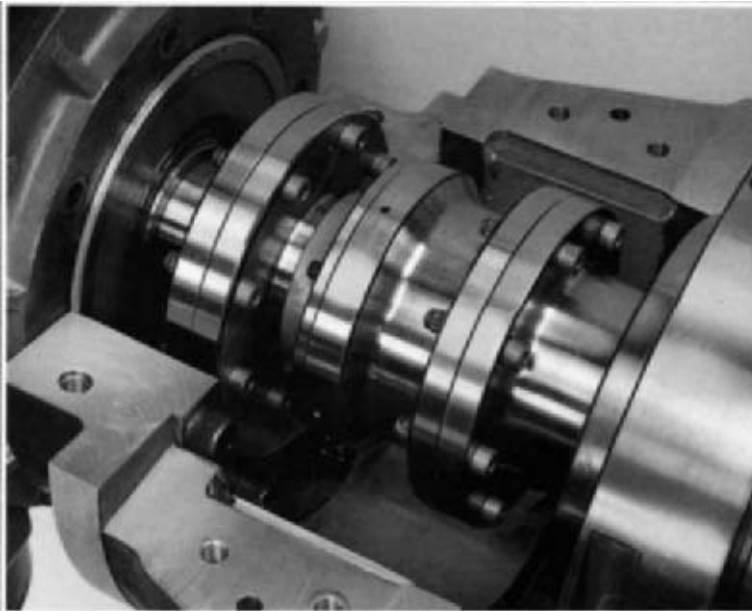
FIG. P-64 Automatic turning gear clutch type MS-8-T installed in gearbox between turning gear and pinion shaft. (Source: MAAG Gear Company.)
