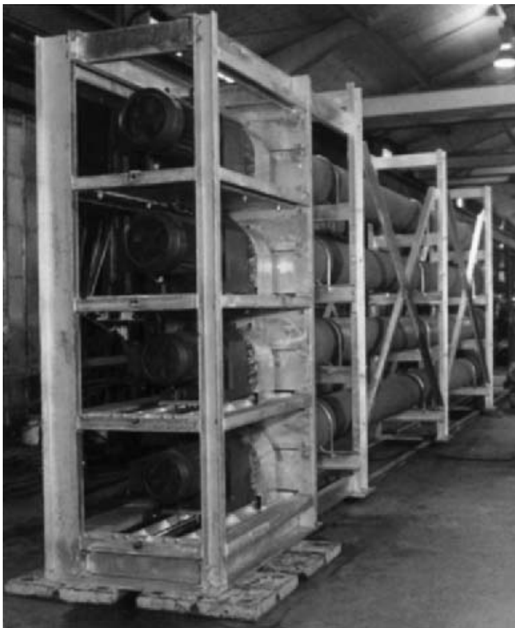
FIG. C-43 Crystallizer for very viscous medium with individual drive gear motors. (Source: Armstrong Engineering Associates.)
