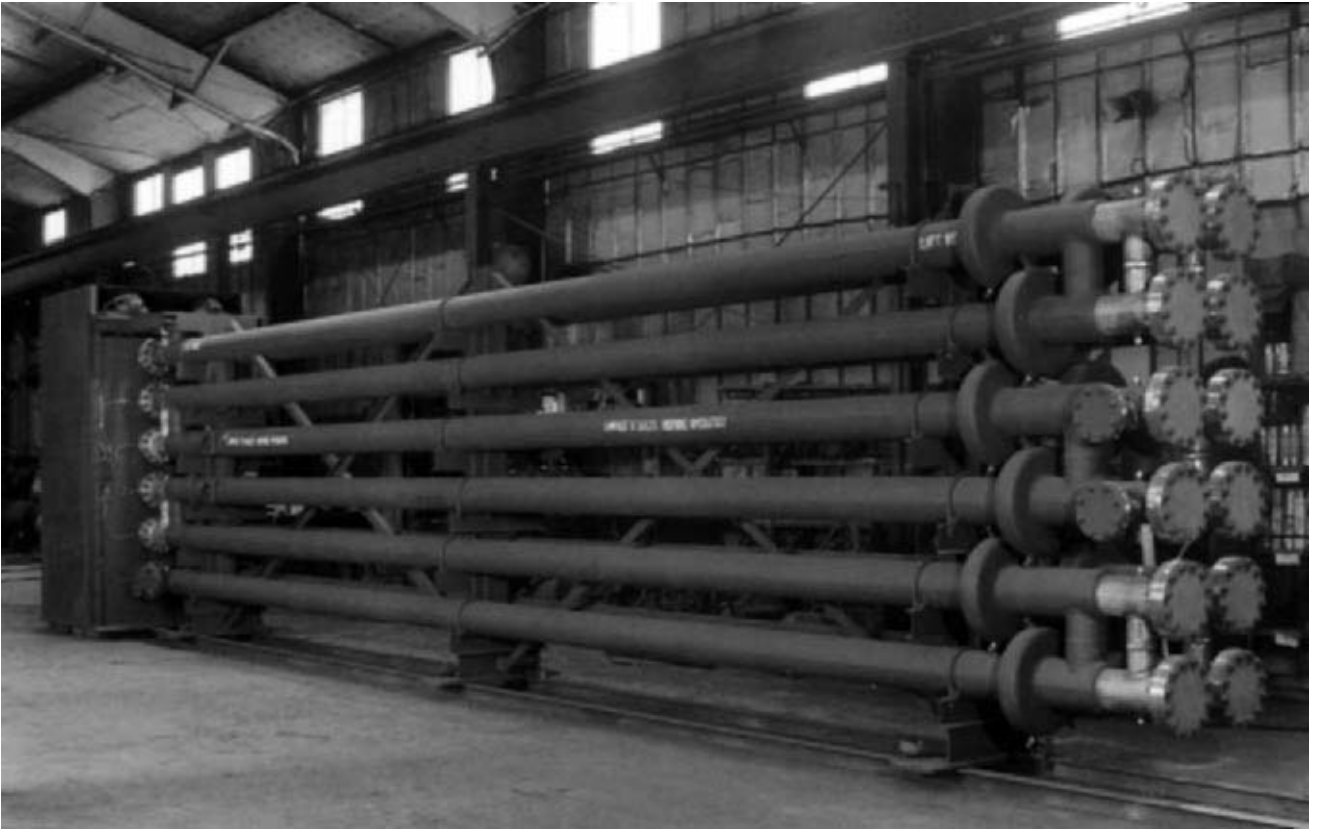
FIG. C-45 Stainless steel process side crystallizer for oligomers formed in fiber processing—three separate process duties are included. (Source: Armstrong Engineering Associates.)
