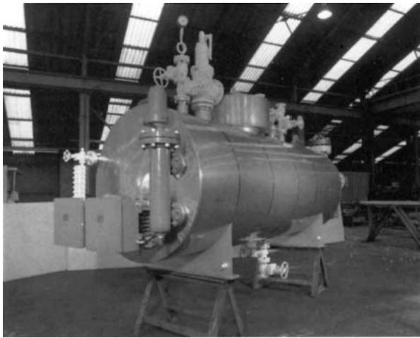
FIG. H-31 Indirect fluid electric vaporizer with controls mounted. High pressure heater of corrosive fluid. Fluid side 3175 psi (223 kg/cm 2 ) design pressure. (Source: Armstrong Engineering Associates.)
