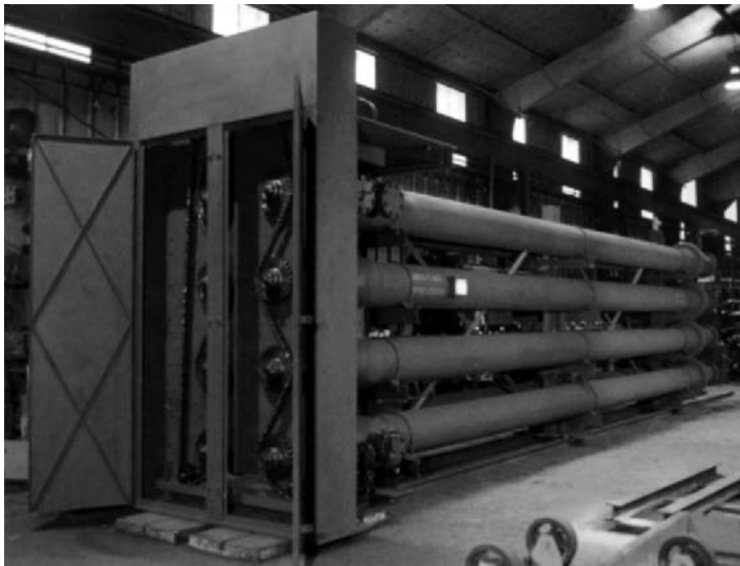
FIG. C-44 Crystallizer for separation of aromatic isomers. (Source: Armstrong Engineering Associates.)
