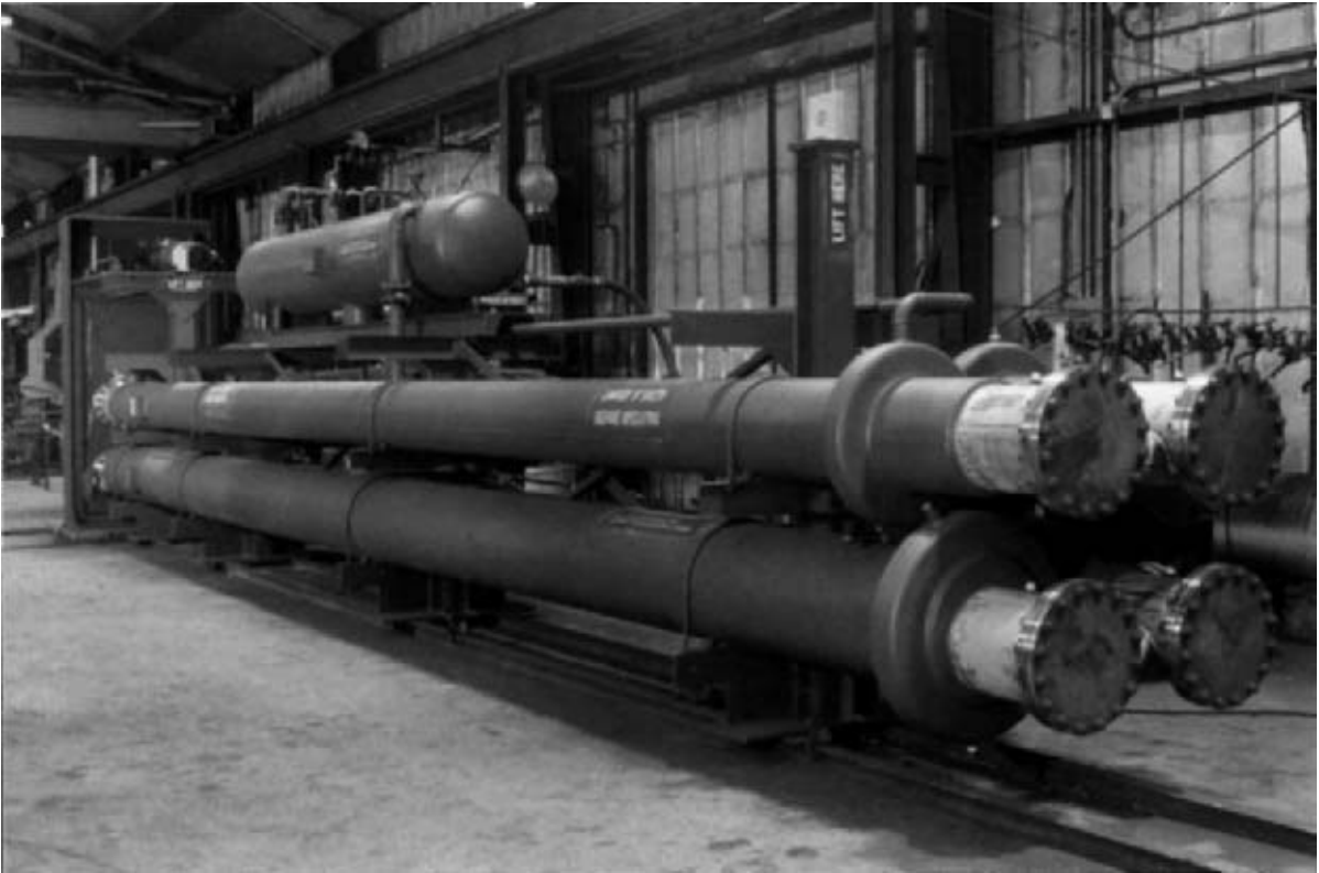
FIG. C-41 Fatty chemical crystallizer with both brine and boiling refrigerant cooling. (Source: Armstrong Engineering Associates.)
