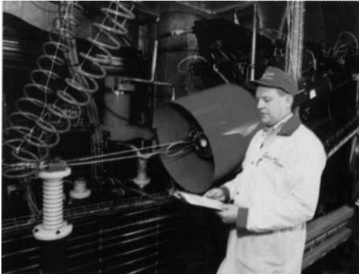
FIG. I-2 Dennis Olson conducts research using a Circe 3 linear accelerator to irradiate meat products at Iowa State University. (Source: "Keeping Food Germ Free.")
