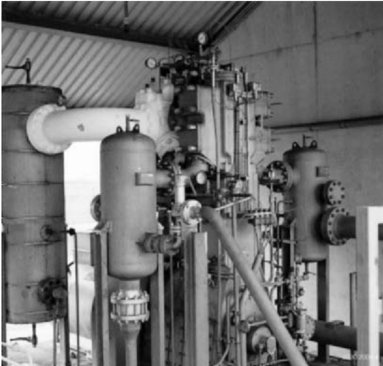
FIG. C-63A Vertical, in-line, reciprocating process compressor, lubricated or oil-free. (Source: Sulzer-Burckhardt.)
