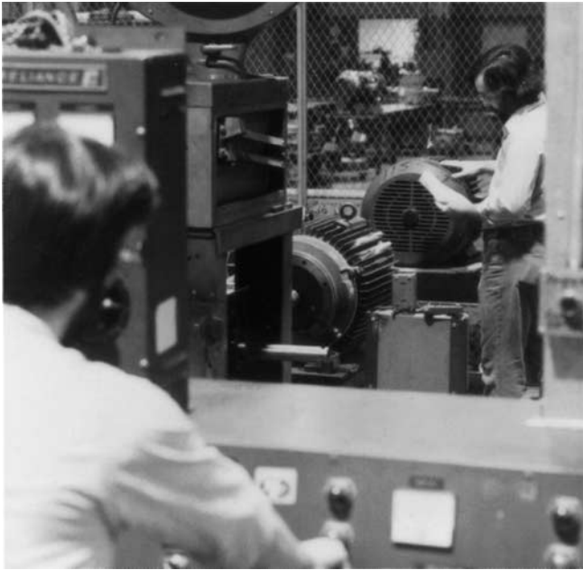
FIG. E-15 Dynamometer testing of Duty Master motors under full-load capacity verifies efficiency and power factors. (Source: Reliance Electric.)
