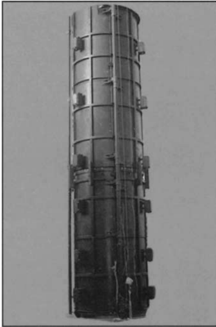
FIG. H-42 1000-kW radiant furnace. Steel vertical vaporizer to heat 1000 kW, 94-in-diameter (2388 mm), 42 ft (12.8 m) overall height. (Source: Armstrong Engineering Associates.)
