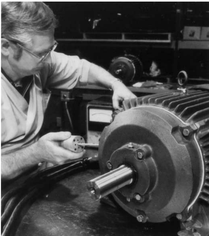
FIG. E-18 Totally assembled motor is vibration tested to NEMA standards. (Source: Reliance Electric.)
