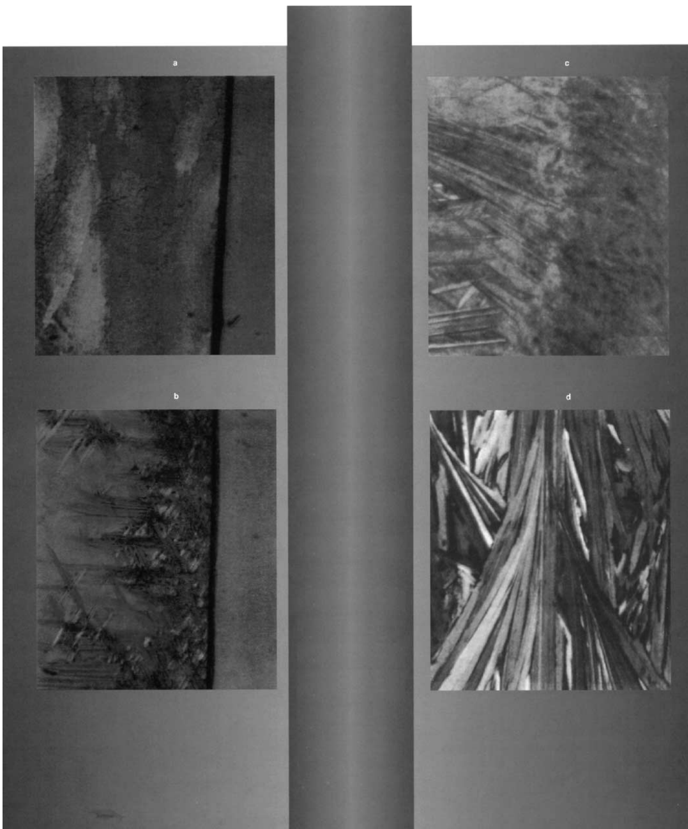
FIG. D-5 Polaroid photographs of frozen TBA-water mixtures with different concentrations of TBA: (a) frozen deionized water, (b) 10% w/w TBA aqueous solution, (c) 50% w/w TBA aqueous solution, (d) 70% w/w TBA aqueous solution. (Source: Kasraian, K., DeLuca, P., Pharmaceutical Research , Vol. 12, No. 4, 1995; permitted by the Plenum Publishing Corporation.)
