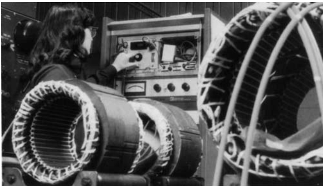
FIG. E-16 Hi-pot testing of wound stator assures electrical integrity per NEMA MG-1 specifications. (Source: Reliance Electric.)
