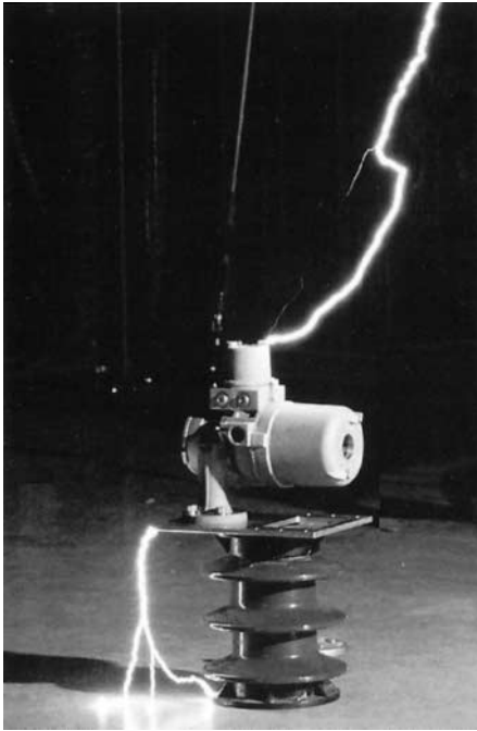
FIG. T-19 Tank gauge under high voltage test. (Source: Enraf.)
