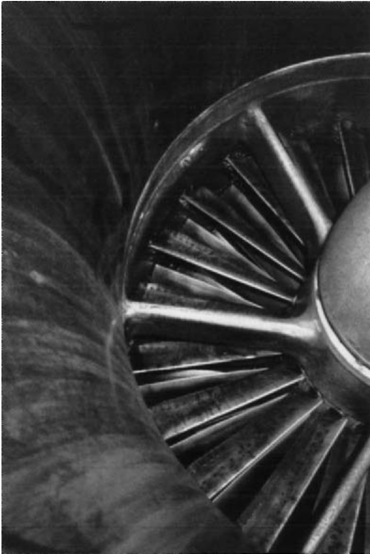
FIG. A-46 Debris in a compressor. (Source: Altair Filters International Limited.)
