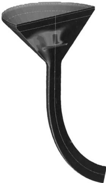
FIG. C-2 Instantaneous solids concentration in a riser, showing how a baffle plate can be used to distribute flow and produce uniform delivery of catalyst to the reactor. (Source: Fluent Inc.)
