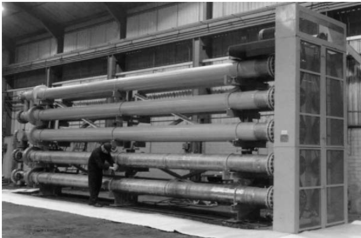
FIG. C-42 Stainless steel process side crystallizer for fatty chemicals—shell side has stainless steel for corrosive coolant in lower section. (Source: Armstrong Engineering Associates.)
