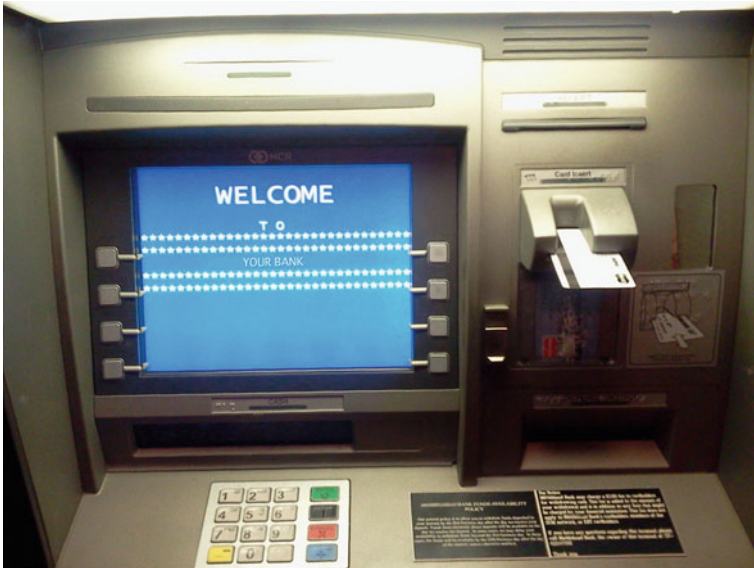
Fig. 6.10 An ATM machine that helps avoid the post-completion error because it does not retain the card. Another way is to return the card before giving money
