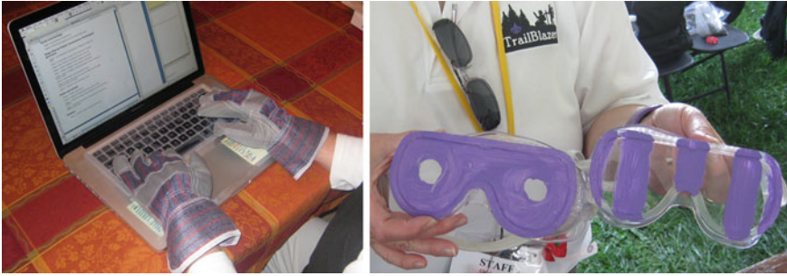
Fig. 3.3 Easy to create modified gloves (they have wooden popsicle sticks in the fingers) and goggles (with paint on them) that give the user restricted hand mobility and restricted vision respectively
