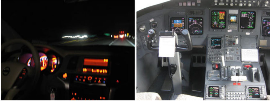
Fig. 5.5 A car dashboard at night ( left ) and a plane's cockpit during the day ( right ). Note similarities and differences, including the use of luminance, color, and some similar interaction devices
