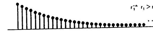
Figure 10.6 With r_1 > r_0 , x[n]r_1^{-n} decays faster with increasing n than x[n]r_0^{-n} . Since x[n] = 0, n < N_1 , this implies that if x[n]r_0^{-n} is absolutely summable, then x[n]r_1^{-n} will be also.
