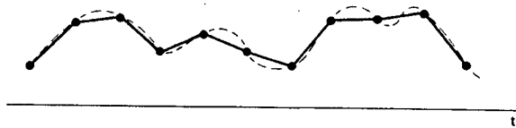
Figure 8.10 Linear interpolation between sample points. The dashed curve represents the original signal and the solid curve the linear interpolation.
