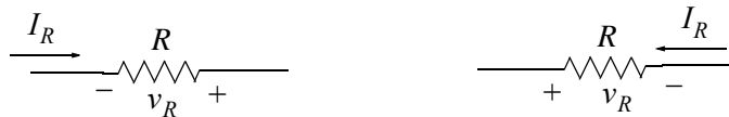
Figure 2.3. Voltage polarity and current direction not in accordance to passive sign convention
