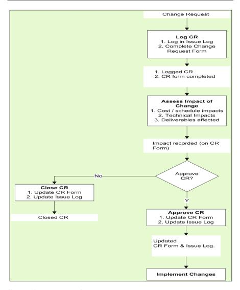
Fig. 5.1 Simple process map for change requests
