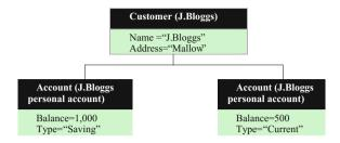
structural relationship that specifies that objects of one thing are connected to objects of another thing. It is indicated by a solid line connecting the same or different classes.
