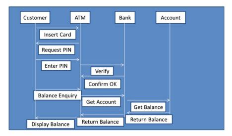
Fig. 14.3 UML sequence diagram for balance enquiry
