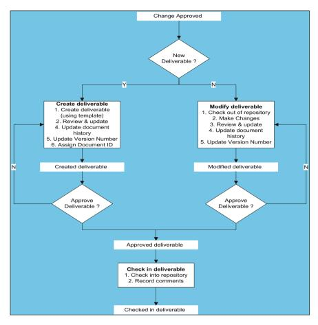
Fig. 5.2 Simple process map for configuration management
