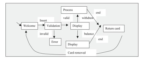
Fig. 14.5 UML state diagram
