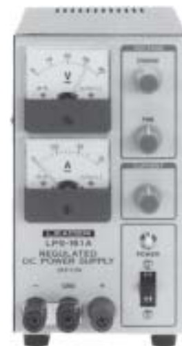
FIG. 2.21 dc laboratory supply. (Courtesy of Leader Instruments Corporation.)
