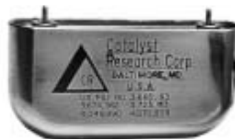
(b) Lithium-iodine pacemaker cell 2.8 V, 2.0 Ah
