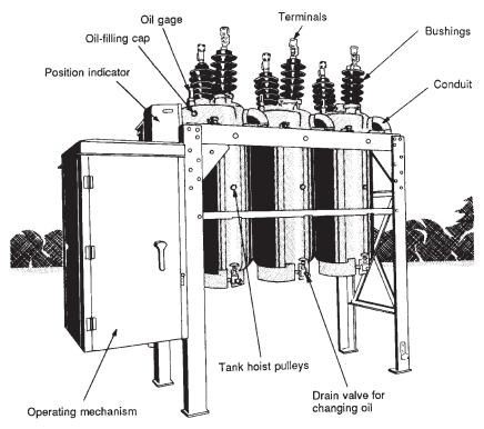
Figure 8-8. Substation oil-circuit breaker.
