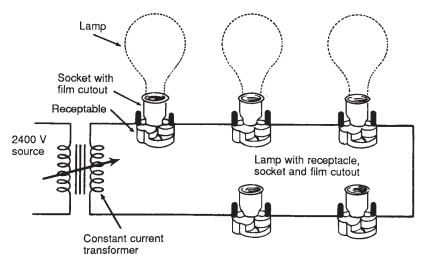
Figure B-7. Series street-lighting circuit.
