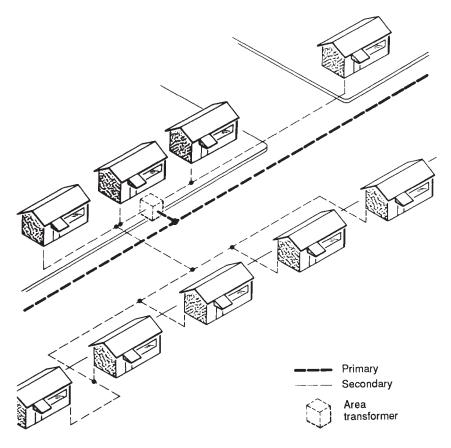
Figure 6-3. Underground residential layout using an area transformer.
