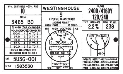
Figure 10-20. Transformer nameplate.
