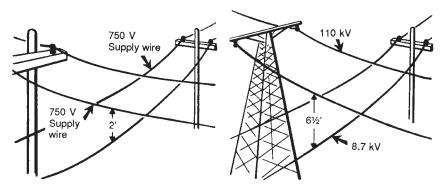
Figure 5-3. Minimum clearances between wires.
