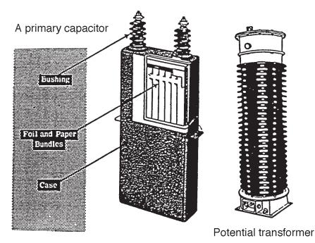
Figure A-5f. More porcelain insulation that may be replaced with polymers.
