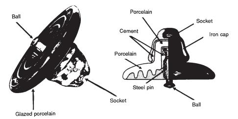
Figure 3-6. Ball and socket-type suspension insulator.
