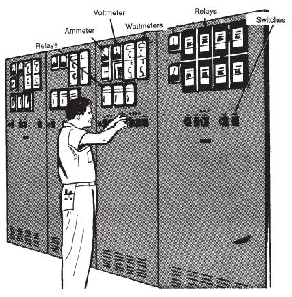
Figure 8-10. Substation switchboard.
