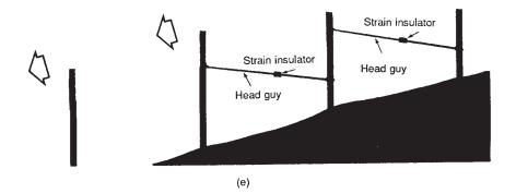
Figure 5-14. (c) Head guys counteract the pull on poles installed on a steep hillside.
