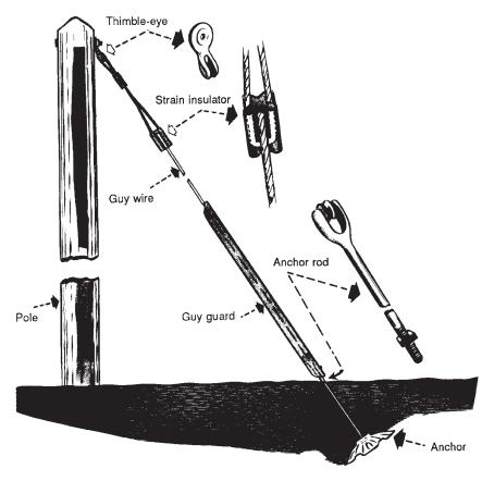
Figure 5-9. Components of an anchor-guy installation.
