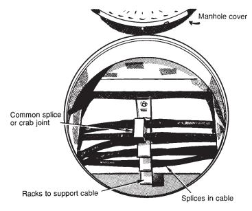
Figure 6-16. Cables spliced and racked in a manhole.
