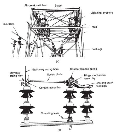
Figure 8-9. Air-break switches. (a) Mounted on a substation rack. (b) Detailed drawing of an air-break switch.
