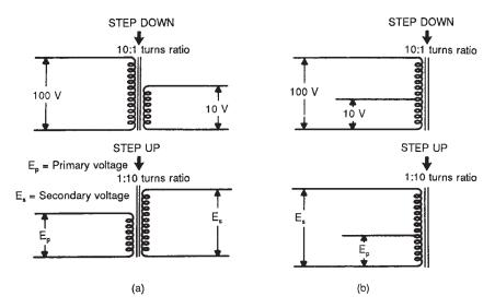
Figure 10-18. Comparison of (a) a conventional transformer and (b) an autotransformer.
