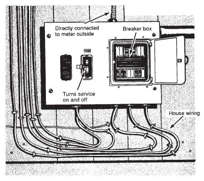
Figure 7-18. An enclosed switch box.
