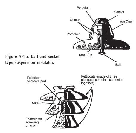
Figure A-1 b. Pin-type insulator.
