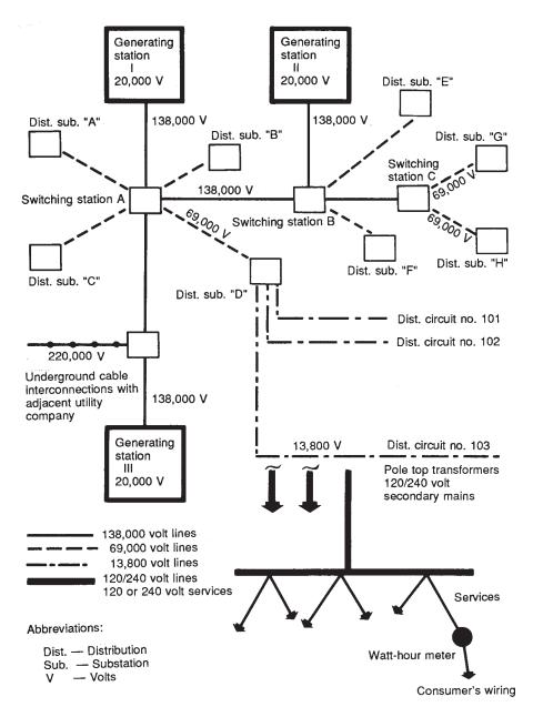
Figure 1-2. Typical transmission and distribution system.
