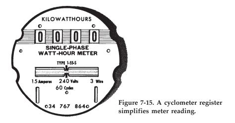
by wheels which indicate numbers directly, making possible the reading of the meter directly, from left to right. This simplifies reading of the meter and takes some of the mystery out of the meter for the average consumer.
