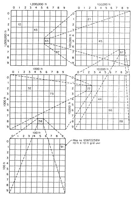
Figure C-1. Development of a grid coordinate system.
