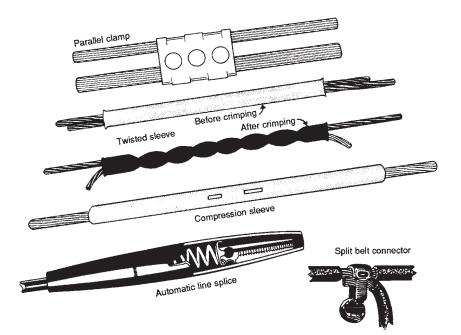
Figure 3-18. Mechanical connectors.
