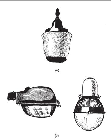
Figure B-15. Diffusing glassware prevents glare, is usually rippled, and comes in many different shapes. (a) Upright fixture (underground wired) and (b) pendant fixtures (overhead wired).
