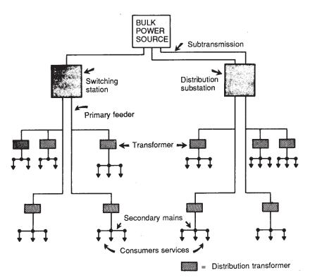
Figure 1-5. Typical distribution system showing component parts.
