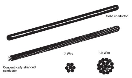
Figure 3-14. Types of conductors. Cross section of stranded conductors.
