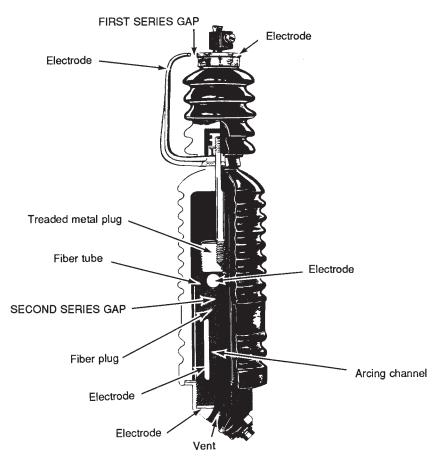
Figure 4-19. Expulsion lightning arrester.
