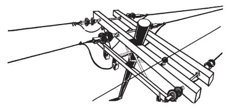
Figure 3-7. How a suspension insulator is used to withstand strain.
