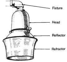
Figure B-14. One type of refractor.
