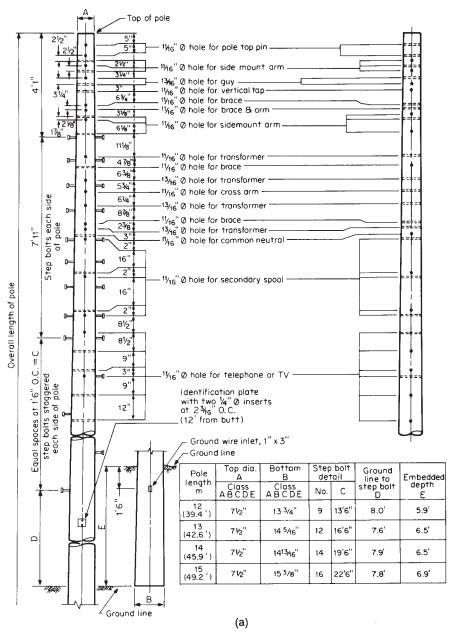
Figure 2-3(a). Reinforced concrete round hollow distribution pole. Pole steps optional. (c) Use of top full upper part of pole. (*Courtesy Centrecon, Inc.*)
