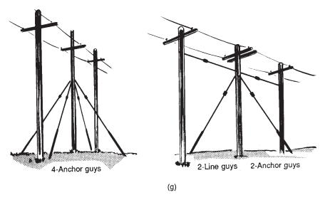
Figure 5-14. (g) Two methods of installing storm guys.
