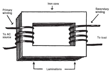
Figure 10-17. The basic transformer.
