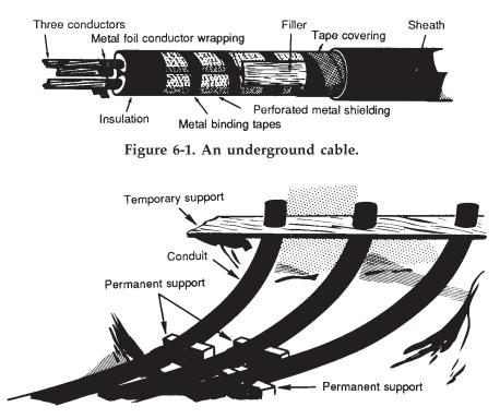
Figure 6-2. Preparing the installation of an underground conduit system.
