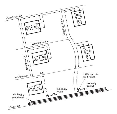
Figure 6-5. Underground residential layout using open-loop construction.
