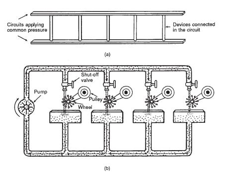
Figure B-4. (a) A multiple circuit is like a ladder. (b) Water analogy of a multiple circuit.
