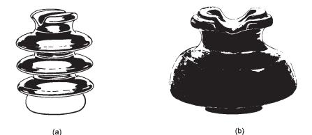
Figure 3-1. Insulators: (a) post type and (b) pin type.
