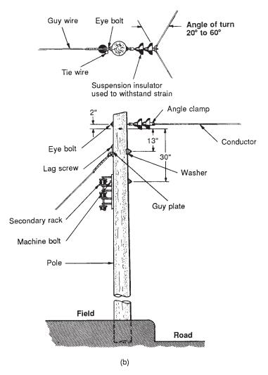
Figure 5-17. (b) Single-conductor pole head,  $20^{\circ}$  to  $60^{\circ}$  angles.
