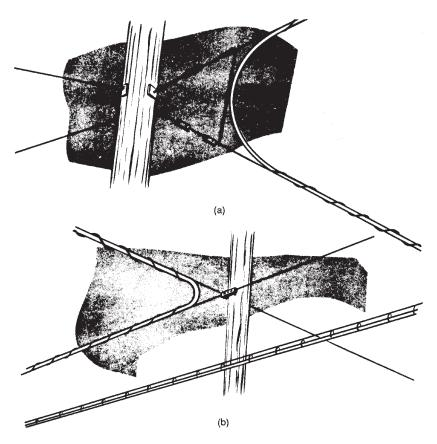
Figure 6-31. Cable "bellied" out around a pole.
