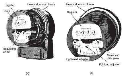
Figure 7-12. Two types of watt-hour meters. (a) A-base and (b) socket S-type.
