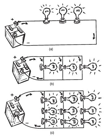
Figure 10-4. Lamps maybe connected to form, (a) a series circuit, (b) a parallel circuit, and (c) a series-parallel circuit.
