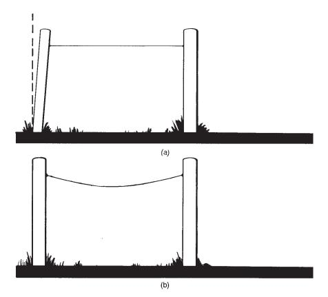
Figure 5-6. Illustration of sag. (a) A taut line causes strain on poles. (b) With a properly sagged line, poles can easily withstand strain.
