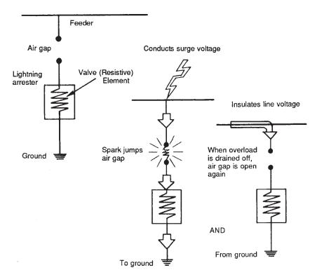
Figure 4-17. Elementary lightning arrester.
