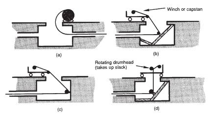
Figure 6-21. Some methods of pulling cable through a duct. (a) Feeding cable into a duct, (b) simple rigging-blocks and wedges, (c) eye imbedded in manhole well, and (d) use of drumhead.
