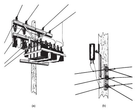
Figure 4-23. Pole-mounted capacitors. (a) Primary and (b) secondary.
