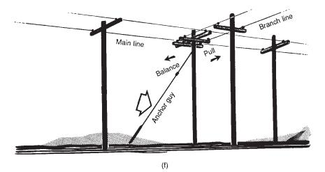
Figure 5-14. (f) A guy is used to counteract the side pull of a branch line connection.
