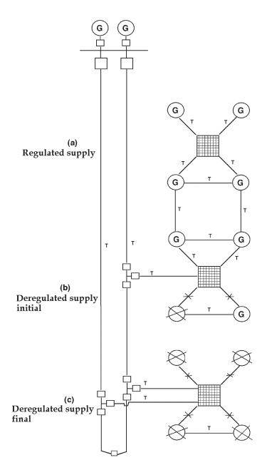
Figure P-1. Simplified schematic diagram of transition from regulated to deregulated supply systems.
