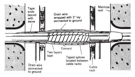
Figure 6-24. Arc-proofing single-conductor cables in a manhole.
