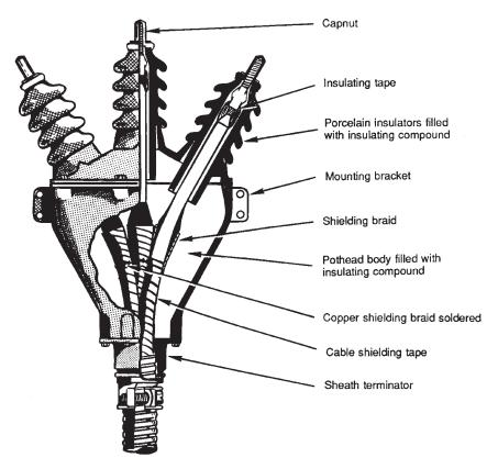
Figure 6-26. Cross section of a pothead.
