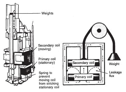
Figure B-9. Constant-current transformer.
