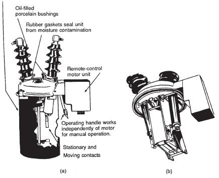
Figure 4-30. An oil switch can be operated manually or by remote control. (a) Cutaway view showing switch in open position. (b) Tank removed showing switch in closed position.
