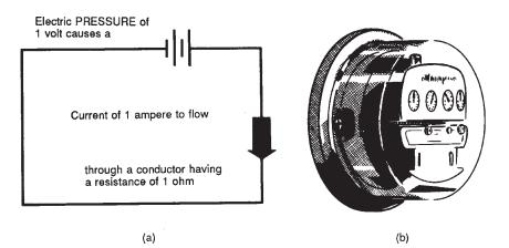
Figure 10-6. Electrical quantities. (a) The power in this circuit is: 1 volt x 1 ampere 1 watt. (b) In 1000 hours, a watt-hour meter would read 1 kilowatt hour.
