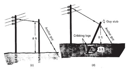
Figure 5-13. (c) Straight and (d) raked stub guy.
