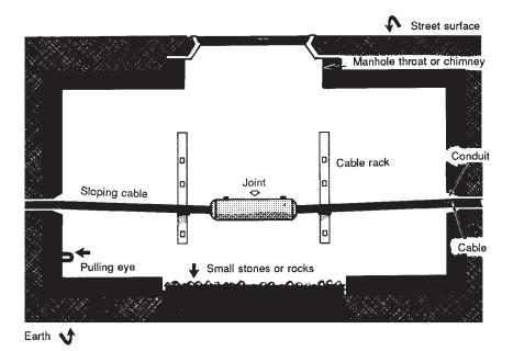
Figure 6-20. Typical manhole with dry well for drainage of rain water.
