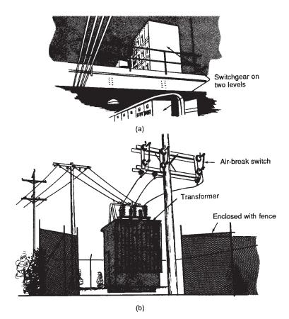
Figure 8-2. Substation types: (a) indoor and (b) outdoor.
