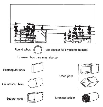
Figure 8-13. Typical types of bus bars in a substation.
