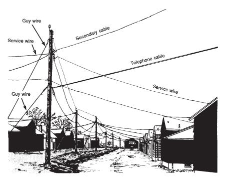
Figure 2-14. Secondary cable installation.
