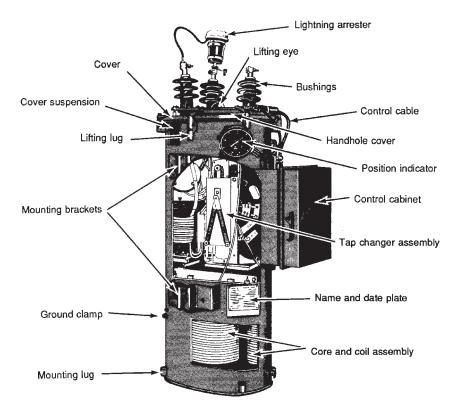
Figure 4-21. Cutaway view of line-voltage regulator.
