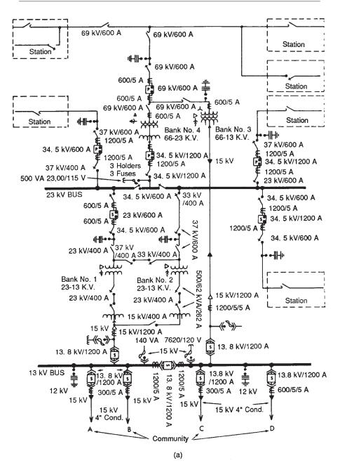
Figure 8-14. (a) Typical arrangement of a substation.
