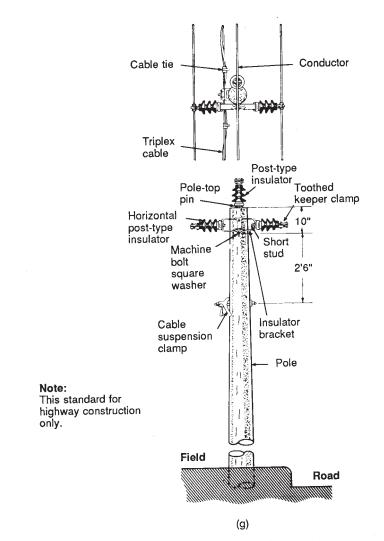
Figure 5-17. (g) Three-conductor pole head,  $0^\circ$  to  $15^\circ$  angles; aimless construction.
