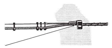
Figure 6-30. A spinning machine wraps wire around a cable and its messenger.
