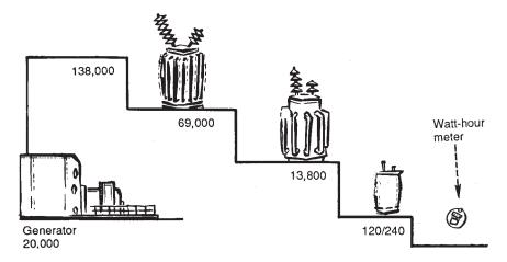
Figure 1-6. Changes in voltage from generator to consumer. All along the journey, voltage is helped down from transmission-line level to a usable level by transformers.
