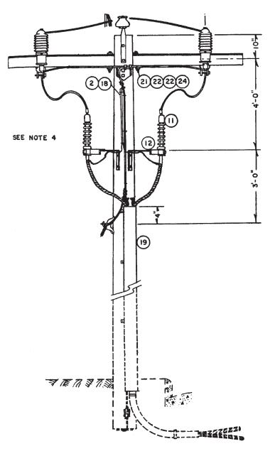
Figure 6-28. Two single-conductor potheads.
