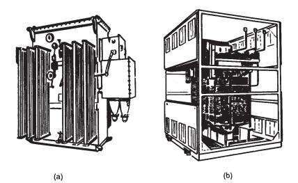
Figure 10-21. Methods of cooling transformers. (a) Oil-filled and (b) air-cooled dry type.
