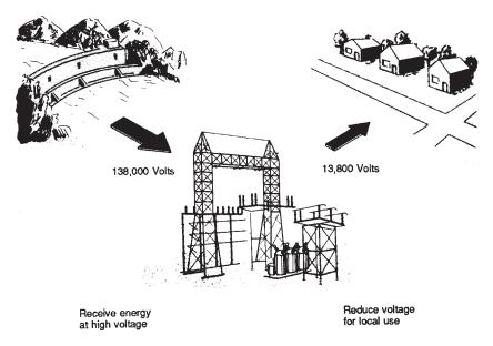
Figure 8-1. Some functions of a substation.
