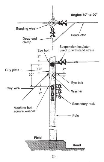
Figure 5-17. (c) Single-conductor pole,  $60^{\circ}$  to  $90^{\circ}$  angles.
