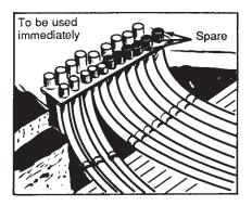
Figure 6-14. Preparing an installation of plastic conduits.
