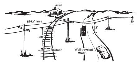
Figure 5-2. Minimum clearances above ground.
