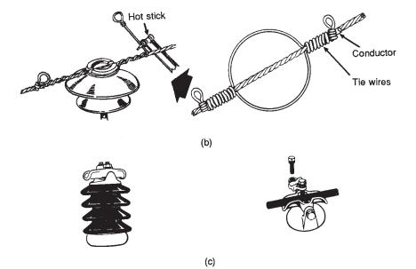
Figure 3-17. (a) Suspension insulators are attached to conductor by a shoe. (b) Tic wire for top groove of pin insulator (straightaway). (c) Clamp-top insulator.
