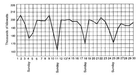
Figure 7-2. Daily peak load for a typical month. How many kilowatts a typical utility company supplies consumers in an average month. Note consistently low peaks on Sunday.
