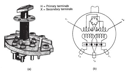
Figure 4-4. Tap changer used to adjust the turns ratio of a transformer. (a) No-load tap change and (b) typical internal wiring of transformer with tap changer.
