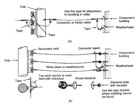
Figure 7-9. Overhead secondary service. (a) Concentric or twisted cable, and (b) open wire.
