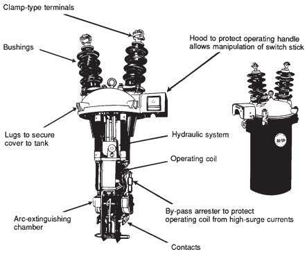
Figure 4-31. Single-phase oil-circuit recloser.
