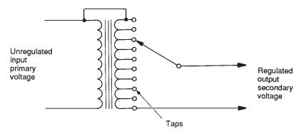
Figure 4-20. Voltage regulator. Schematic diagram of tap-changingunder load (TCUL) regulator.
