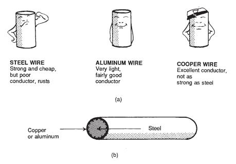
Figure 3-13 (a). Comparison of metal conductors. (b) Copperweld or Alumoweld conductor used for rural distribution and guy wires.
