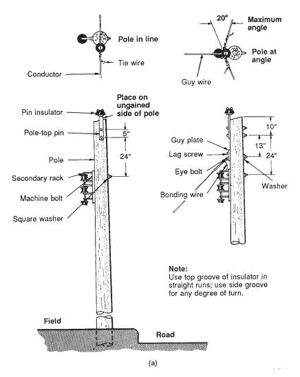
Figure 5-17. Typical construction standards for a primary line assembly. (a) Single-conductor pole head,  $0^{\circ}$  to  $20^{\circ}$  angles.
