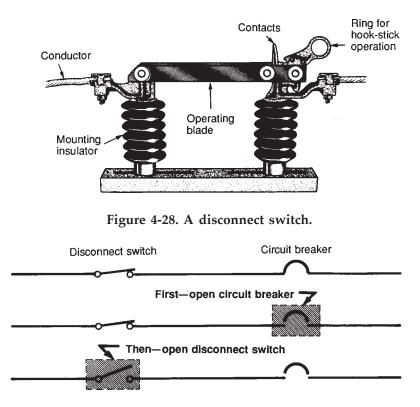
Figure 4-29. The disconnect switch is never opened under load.
