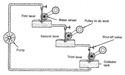
Figure B-6. Water analogy of a series circuit.
