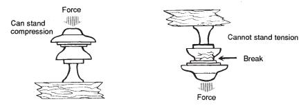
Figure 3-2. How porcelain reacts to compression and tension forces.
