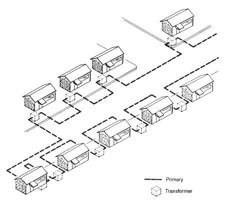
Figure 6-4. Underground residential layout using individual transformers.
