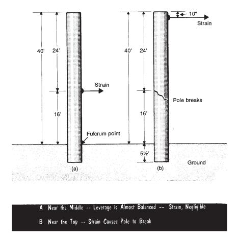
Figure 2-6. Effects of applying loads at different points on a pole. (a) Near the middle, leverage is almost balanced and strain is negligible. (b) Near the top, strain causes the pole to break.
