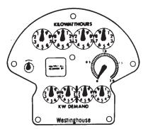
available for checking, until the meter is next read, when the lever or plunger which returns the "floating" hand to zero causes the new maximum demand to be added to the original reading: the new reading will then be greater than the previous one by the current period's maximum demand.
