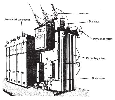
Figure 8-6. A substation transformer.
