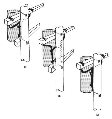
Figure 4-7. Hanger-iron method of mounting distribution transformers on poles. (a) T-shaped hanger iron using two crossarms. (b) C-shaped hanger-iron designed to hold larger transformers. (c) For smaller transformers, a T-shaped hanger-iron one crossarm and a kicker are sufficient.
