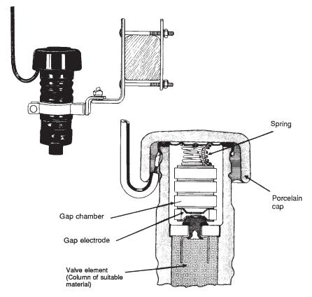
Figure 4-18. Valve lightning arrester.
