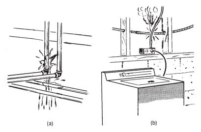
Figure 1-8. The danger of high voltages. (a) Pipe rupturing-water spills over adjacent areas; (b) Rupture of cable insulation causes arcing to other wires-sometimes causing flame.
