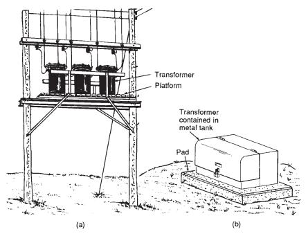
Figure 4-8. Mounting of distribution transformers. (a) Platform mounted and (b) pad mounted.
