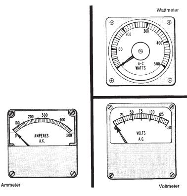
Figure 8-11. Indicating instruments used in a substation.
