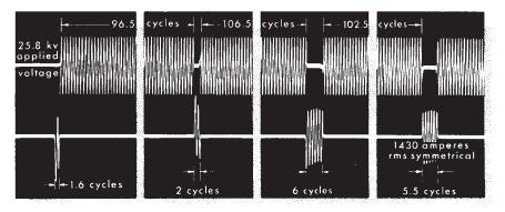
Figure 4-32. Oscillogram showing example of recloser operation.
