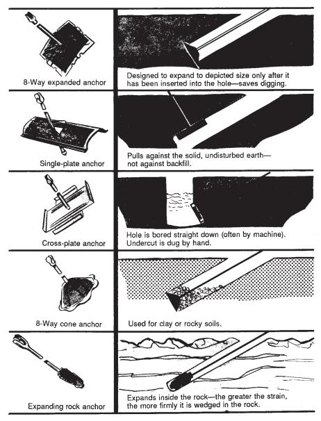
Figure 5-12. Guy anchors and their installation.
