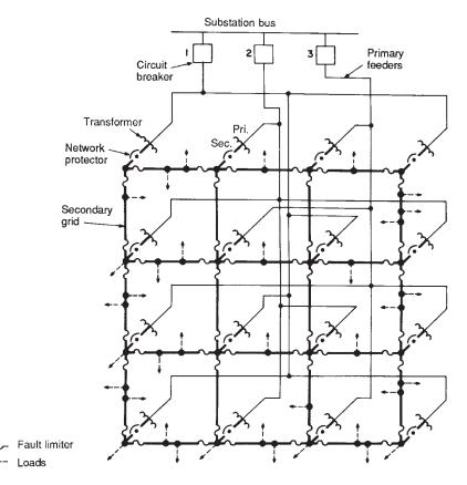
Figure 6-7. Secondary underground network. Protector switches are used to prevent feedback.
