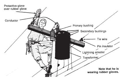
Figure 3-15. Lineworker working on line conductor.
