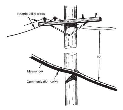
Figure 5-16. Joint construction of telephone and electric cables.
