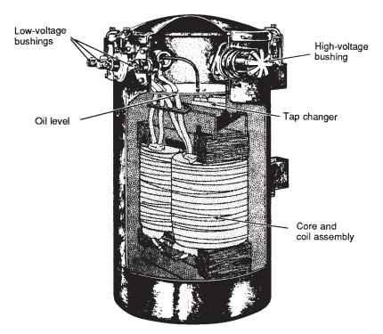
Figure 4-2. Basic components of a distribution transformer.
