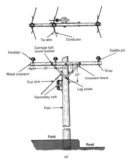
Figure 5-17. (e) Three-conductor pole head, medium angles.
