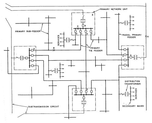
Figure 9-4. Typical primary-network arrangement using breakers.
