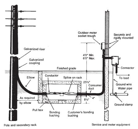
Figure 7-10. Layout for a typical underground service.
