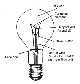
Figure B-16. Basic construction of the incandescent lamp,
