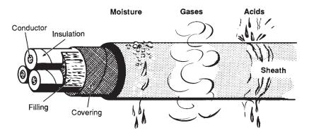
Figure 6-10. Underground cable protection provided by the sheath.
