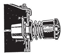
Figure A-5(b). Sidewall-mounted bushing.
