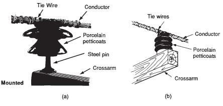
Figure 3-4 (a). Pin and (b) post-type insulators.
