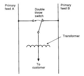
Figure 6-6. Use of throw-over switch for extra reliability.
