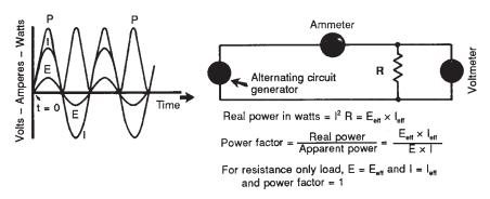
Figure 10-10. Power in an ac circuit. Circuit containing resistance only.
