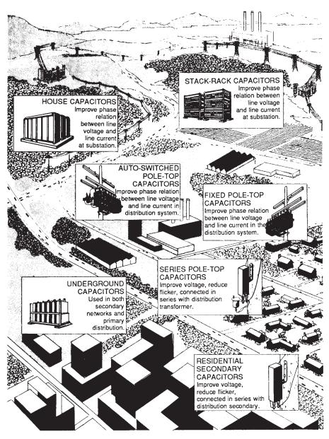
Figure 4-24. How capacitors are used.
