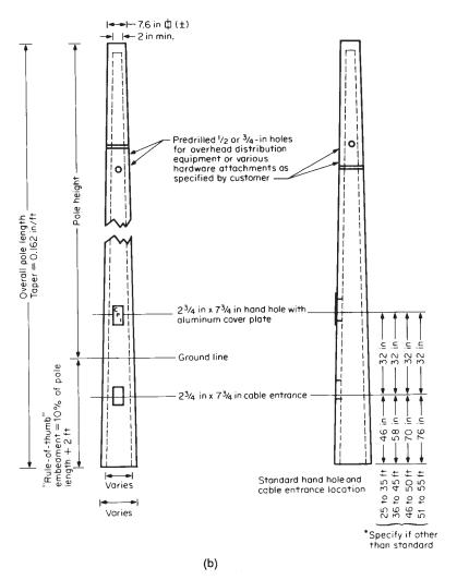
Figure 2-3(b). Reinforced concrete square hollow distribution pole. (*Courtesy Concrete Products, Inc.*)
