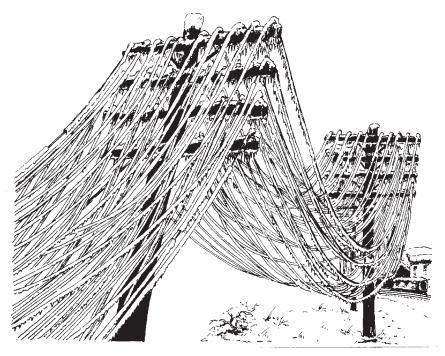
Figure 2-5. Ice-laden conductors.
