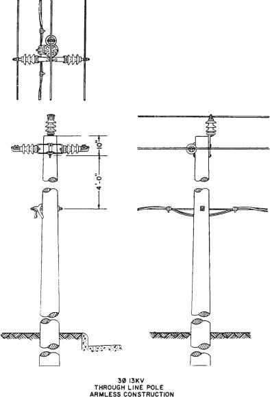
ARMLESS CONSTRUCTION 20KV INSULATORS
