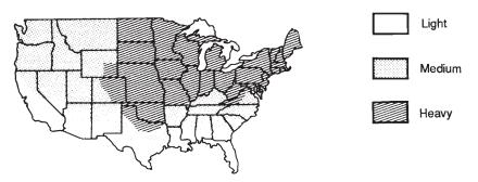
Figure 2-7. Wind and ice load specifications. Map shows territorial division of the United States with respect to wind and ice loading of overhead lines. Alaska is in the heavy zone and Hawaii is in the light. (*National Electric Safety Code*)
