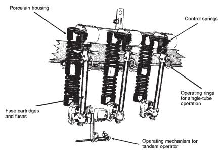
Figure 4-15. Repeater-type fuse cutout.
