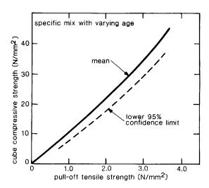
Figure 4.30 Typical pull-off/strength correlation for natural aggregate (based on ref. 106).
