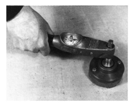
Figure 4.17 Torquemeter loading method.
