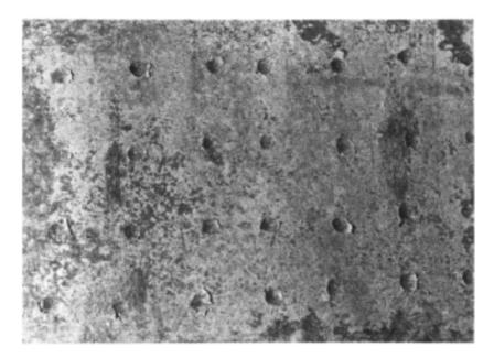
Figure 2.10 Surface damage on green concrete.
