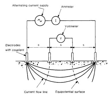
**Figure 7.10** Four-probe resistivity test.
