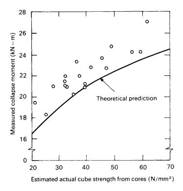
**Figure 6.20** Measured vs. calculated collapse moments for prestressed concrete beams.
