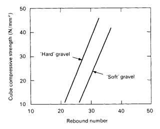
Figure 2.5 Comparison of hard and soft gravels—vertical hammer.
