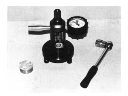
Figure 4.27 'Hydrajaws' tripod equipment.
