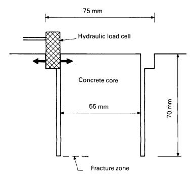
Figure 4.32 Break-off method.
