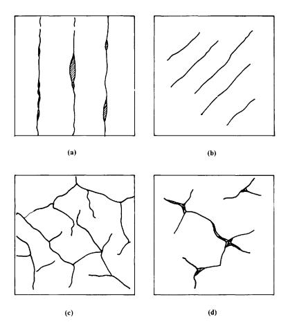
**Figure 1.2** Some typical crack types: (a) reinforcement corrosion; (b) plastic shrinkage; (c) sulphate attack; (d) alkali/aggregate reaction.
