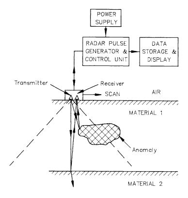
Figure 8.2 Investigation of sub-surface anomaly using radar.
