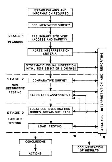
Figure 1.1 Typical stages of test programme (based on ref. 17).
