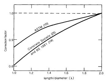
Figure 5.5 Length/diameter ratio influence (based on refs 25, 114 and 115).
