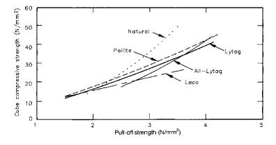
Figure 4.31 Typical strength correlations for lightweight aggregates.
