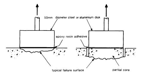
**Figure 4.25** Pull-off method—surface and partially cored.
