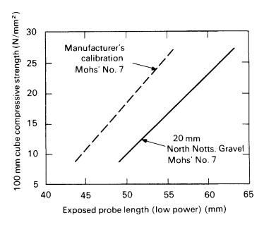
Figure 4.6 Comparison of calibrations (based on refs 76 and 80).
