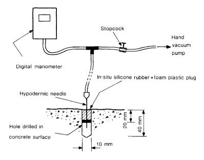
Figure 7.18 Modified Figg air permeability test (based on ref. 216).
