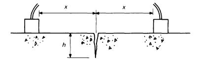
Figure 3.21 Crack depth measurement.
