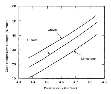
**Figure 3.8** Effect of aggregate type (all concretes similar apart from aggregate type) (based on ref. 62).
