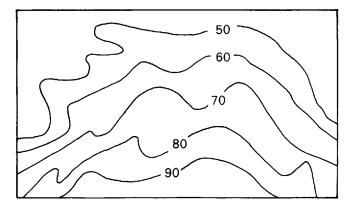
Figure 1.5 Typical relative percentage strength contours for a wall.
