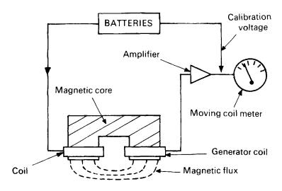
Figure 7.2 Typical simple covermeter circuitry.
