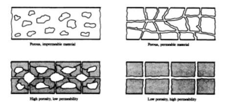
Figure 7.15 Porosity and permeability (based on ref. 205).
