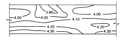
**Figure 3.20** Typical pulse velocity beam contours (km/s).
