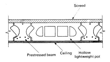
Figure 6.1 Beam and pot construction.
