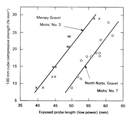
**Figure 4.5** Typical low power strength calibration (based on ref. 80).
