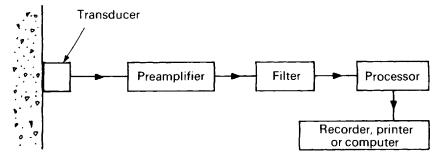
Figure 8.14 Acoustic emission-equipment.
