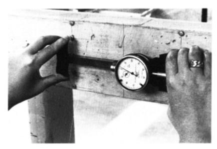
Figure 6.15 Photo of Demec gauge.
