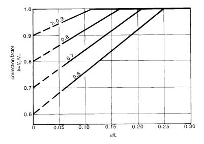
Figure 3.17 Correction factors for bars parallel to pulse path [a>2b] (based on ref. 58).
