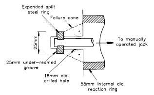
Figure 4.24 Capo test configuration.
