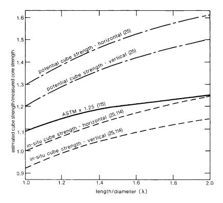
Figure 5.6 Effect of calculation method (baed on refs 25, 114 and 115).
