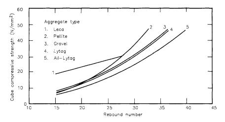
Figure 2.6 Comparison of lightweight aggregates (based on ref. 24).
