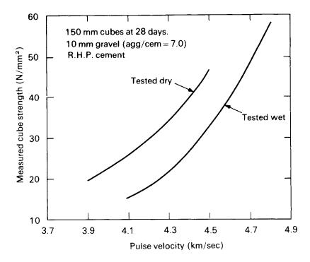
Figure 3.13 Effect of moisture conditions (based on ref. 65).
