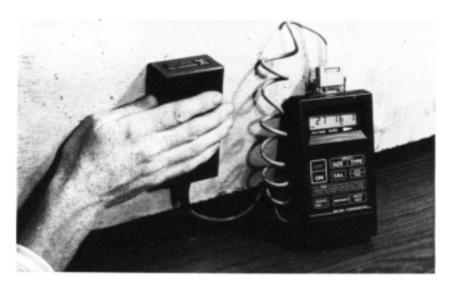
Figure 7.5 Microcovermeter.
