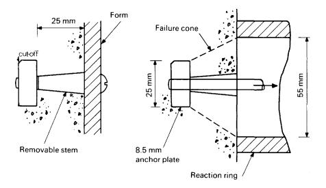
Figure 4.9 Lok-test insert.
