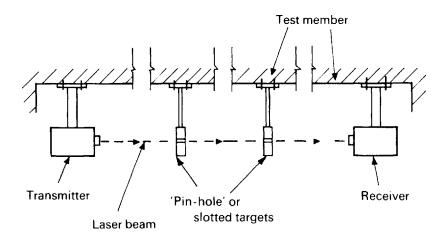
Figure 6.13 Laser beam for long-term monitoring.
