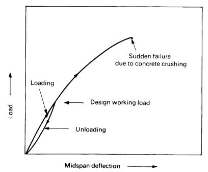
Figure 6.19 Load/deflection curve for typical over-reinforced prestressed beam.
