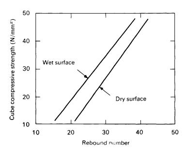
Figure 2.7 Influence of surface moisture condition—horizontal hammer (based on ref. 49).
