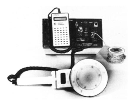
Figure 7.9 'Wheel' half-cell equipment.
