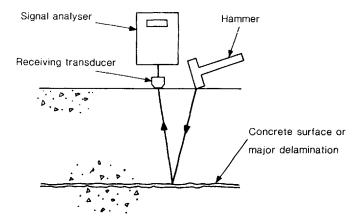
**Figure 8.6** Instrumented delamination device.
