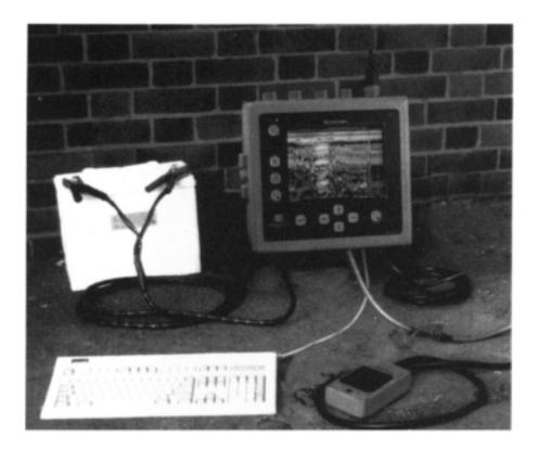
Figure 8.4 Digital impulse radar system.
