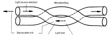
Figure 6.14 Stranded optical fibre (based on ref. 146).
