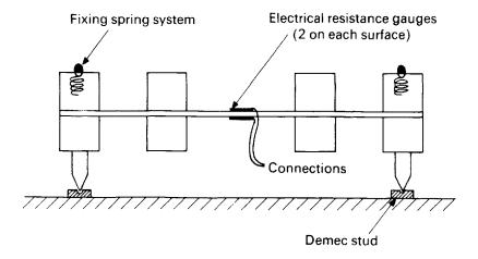
Figure 6.16 Portal strain transducer.
