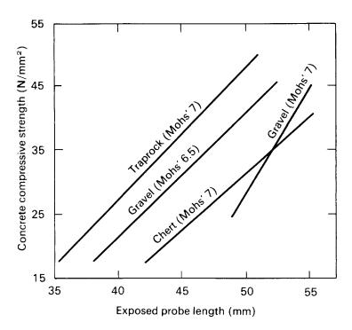
Figure 4.7 Influence of aggregate type and proportions (based on ref. 50).
