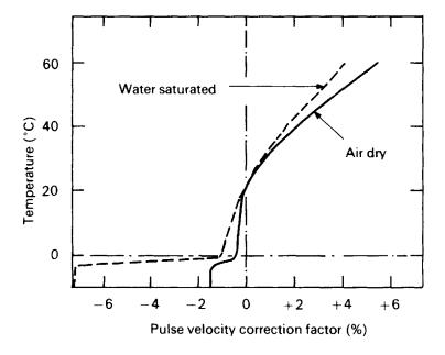
Figure 3.11 Effect of temperature (based on ref. 64).
