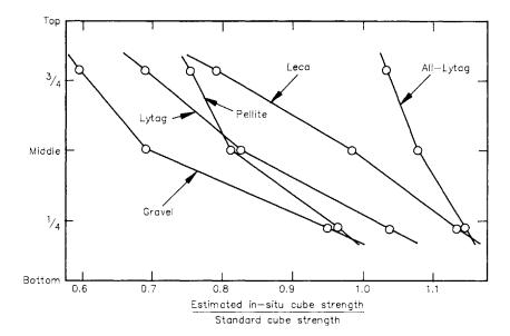
**Figure 1.6** Average relative strength distributions within beams of different concrete types (based on ref. 24).
