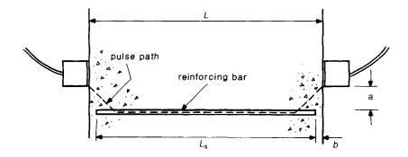
Figure 3.15 Reinforcement parallel to pulse path.
