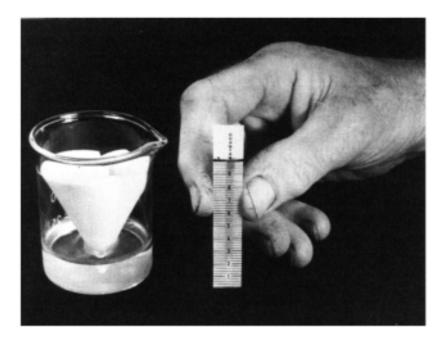
Figure 9.3 'Quantab' chloride test.
