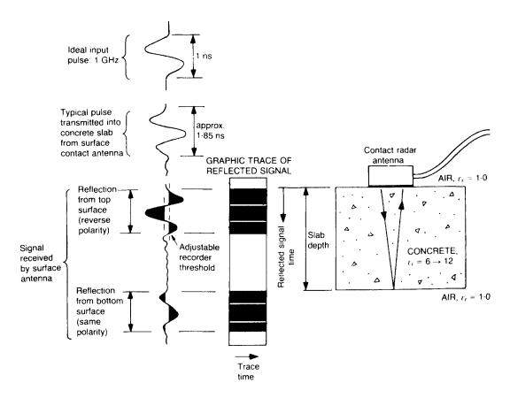
**Figure 8.3** Radar reflections from a concrete slab (based on ref. 241).
