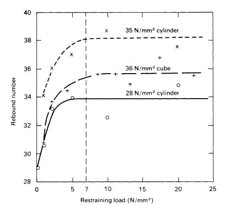
Figure 2.8 Effect of restraining load on calibration specimen (incorporating data from ref. 50).
