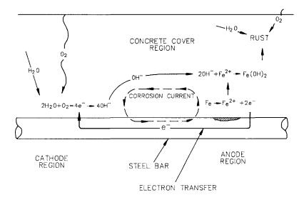
**Figure 7.1** Basic corrosion process of steel reinforcement in concrete.
