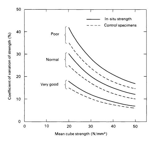
Figure 1.9 Coefficient of variation of test results related to concrete strength.
