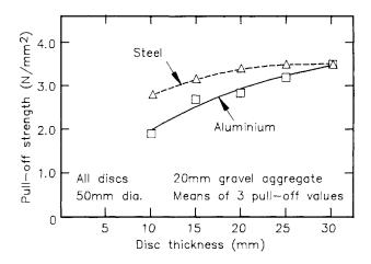
Figure 4.28 Effects of disk type and thickness (based on ref. 105).
