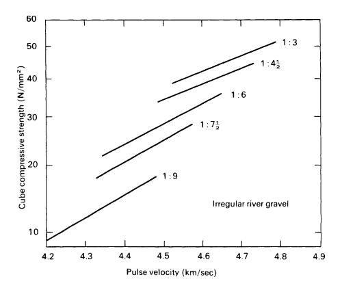
Figure 3.10 Effect of aggregate proportions (based on ref. 62).
