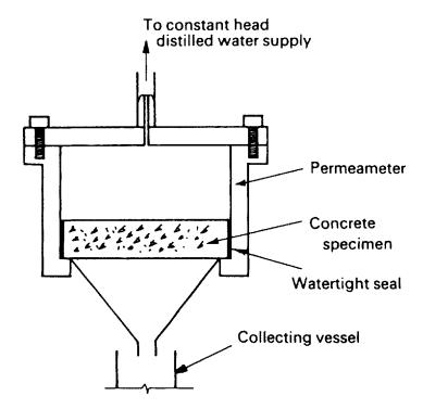
Figure 7.21 Typical permeability equipment.
