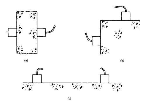
Figure 3.4 Types of reading, (a) Direct; (b) semi-direct; (c) indirect.
