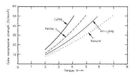
**Figure 4.21** Comparison of calibration curves for lightweight aggregates (torquemeter method) (based on ref. 24).
