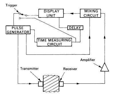
Figure 3.1 Typical UPV testing equipment.
