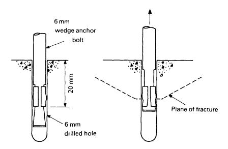
Figure 4.15 Internal fracture test.
