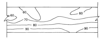
Figure 1.4 Typical relative percentage strength contours for a beam.
