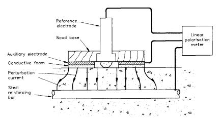
Figure 7.12 Linear polarization resistance measurement.
