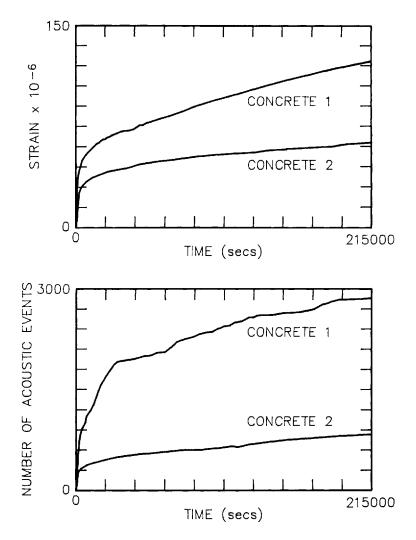
**Figure 8.16** Acoustic emission tests on creep specimens (based on ref. 289).
