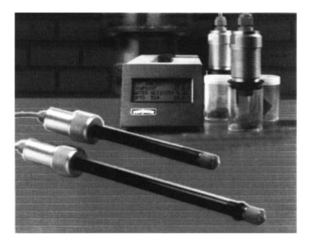
Figure 7.14 Chilled mirror relative humidity meter (photograph by courtesy of Protimeter Plc).
