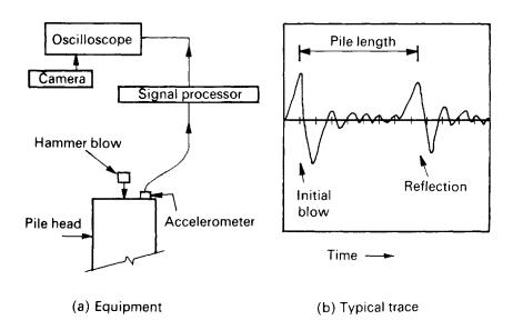
**Figure 8.7** Pulse-echo method; time domain measurement.
