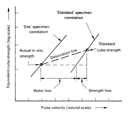
Figure 3.14 Desiccation line method (based on ref. 33).
