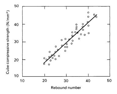
Figure 2.9 Typical rebound number/compressive strength calibration chart.
