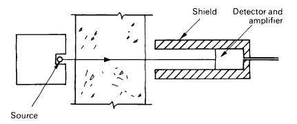
Figure 8.12 Direct radiometry.
