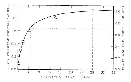
**Figure 8.20** Relative strength *vs.* equivalent age (based on ref. 294). (Note that the left scale is based on the final long-term strength and the right scale on the 28 day strength).
