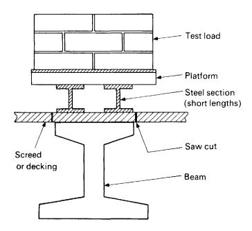
**Figure 6.3** Test load concentrated on beam.
