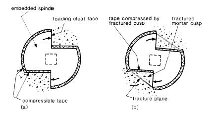
**Figure 4.33** Stoll tork test (based on ref. 113). (a) Before fracture, (b) After fracture.
