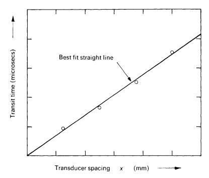
Figure 3.6 Indirect reading—results plot.
