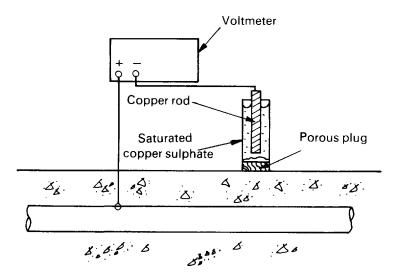
Figure 7.6 Reinforcement potential measurement.
