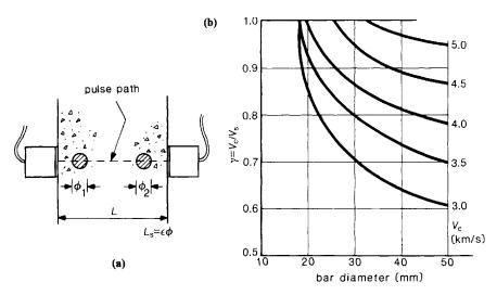
**Figure 3.19** Reinforcement transverse to pulse path (based on ref. 58). (a) Path through transverse reinforcement, (b) Bar diameter/velocity ratio.
