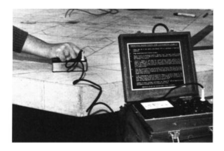
Figure 7.3 Typical simple covermeter.
