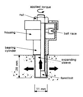
Figure 4.22 ESCOT expanding sleeve test system (based on ref. 99).
