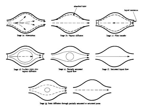
Figure 7.16 Movement of water and ions within concrete pore (based on ref. 205).
