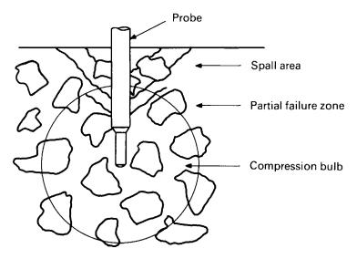
Figure 4.4 Compaction bulb.
