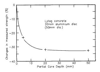
**Figure 4.29** Effects of partial coring (based on ref. 105).
