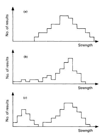
**Figure 1.8** Typical histogram plots of in-situ test results: (a) uniform supply; (b) poor construction; (c) two sources.
