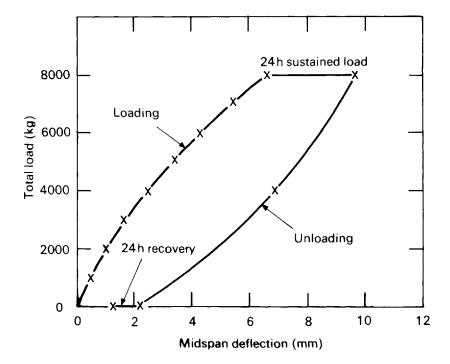
Figure 6.12 Typical load test result plot.
