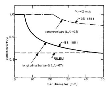
Figure 3.18 Typical correction factors.
