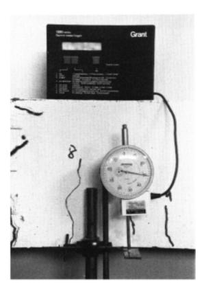
**Figure 6.8** Dial gauge/displacement transducer with portable battery-powered logger.
