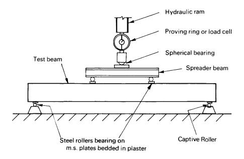
Figure 6.18 Laboratory beam load test arrangement.
