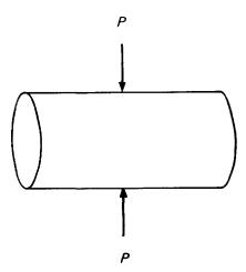
Figure 5.3 Point load test.
