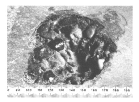
Figure 4.8 Surface damage caused by probe removal.
