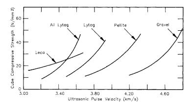
Figure 3.9 Comparison of lightweight and gravel aggregates (based on ref. 27).
