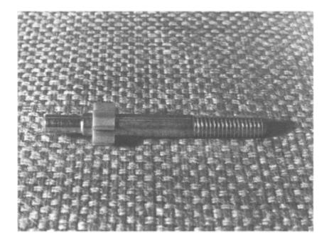
**Figure 4.1** Penetration resistance test probe.
