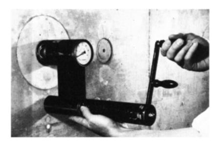
Figure 4.10 Lok-test equipment (photograph by courtesy of Lok-test Aps.).
