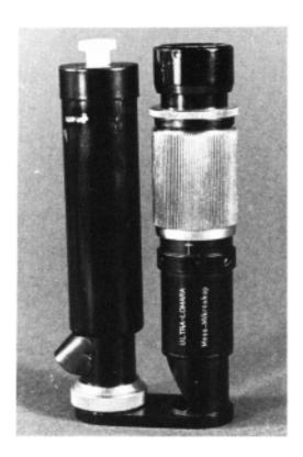
Figure 6.10 Crack microscope.
