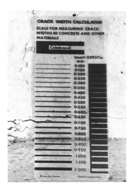
Figure 6.11 Crack width measurement scale.
