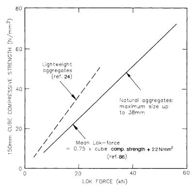
Figure 4.11 Typical Lok-test calibration chart (based on refs 24 and 86).
