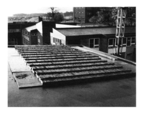
Figure 6.5 Test load on roof slab using bricks (photograph by courtesy of Tysons Contractors Ltd.).
