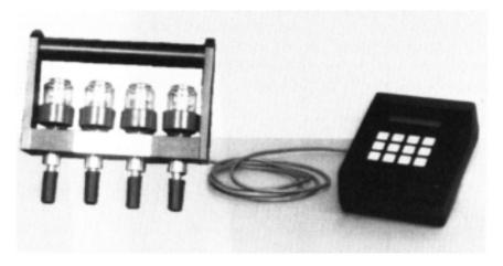
Figure 7.11 Four-probe resistivity equipment.
