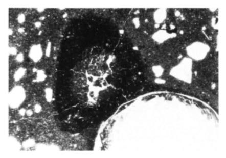
**Figure 9.5** Photomicrograph of alkali-silica reaction (photograph by courtesy of Professor E. Poulsen). Note: An opaline chert particle is seriously affected by ASR, with cracks radiating into the surrounding paste. The air void in the lower right hand corner is also partially filled with gel.
