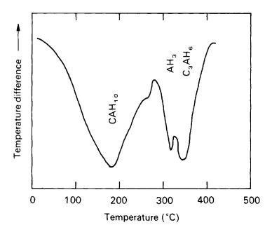
**Figure 9.7** Typical differential thermal analysis trace (based on ref. 334).
