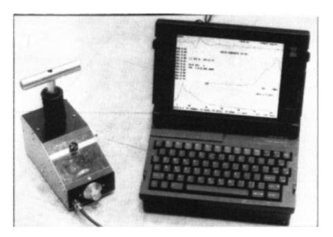
Figure 8.10 DOCter impact-echo apparatus.
