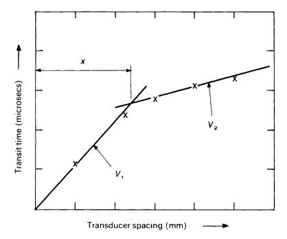
Figure 3.22 Layer thickness measurement.
