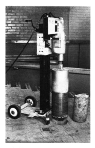
Figure 5.1 Core cutting drill.
