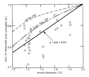
Figure 5.7 Length/diameter ratio for small cores (based on refs 25, 115 and 127).
