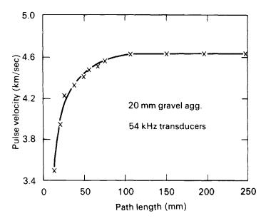
Figure 3.12 Effect of short path length (based on ref. 65).
