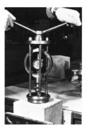
Figure 4.18 Proving ring loading method.
