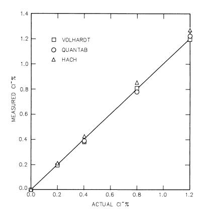
Figure 9.4 Comparison of chloride analysis results.
