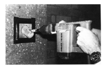
Figure 9.1 Field collection of drill dust sample.
