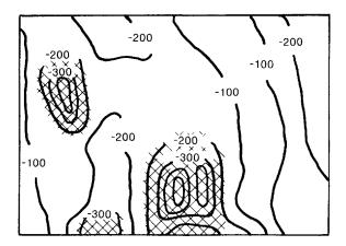
Figure 7.7 Typical half-cell potential contours (based on ref. 159).; zones requiring further investigation.
