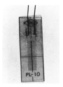
Figure 6.17 Electrical resistance strain gauge.
