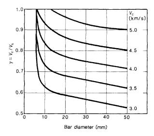
**Figure 3.16** Relationship between bar diameter and velocity ratio for bars parallel to pulse path (based on ref. 58).
