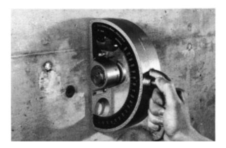
Figure 2.4 Pendulum hammer.
