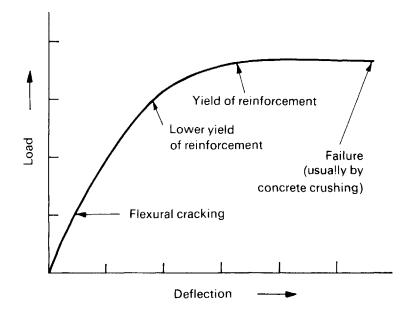
**Figure 6.2** Typical load deflection curve for under-reinforced beam.
