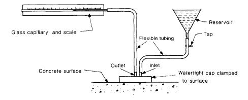
Figure 7.17 Initial surface absorption test.
