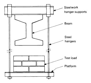
Figure 6.4 Test load arrangement for purlins.
