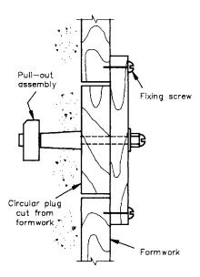
Figure 4.12 Arrangement for formwork stripping time tests.
