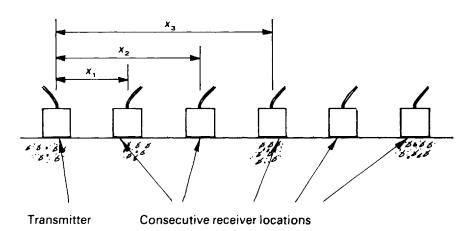
Figure 3.5 Indirect reading—transducer arrangement.
