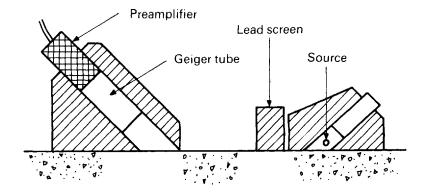
Figure 8.13 Backscatter radiometry.
