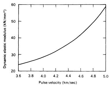
Figure 3.7 Pulse velocity vs. dynamic elastic modulus (based on ref. 58).
