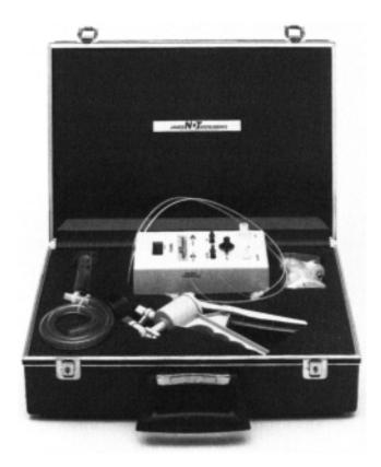
Figure 7.19 Automatic Figg test equipment (photograph by courtesy of James Instruments Inc).
