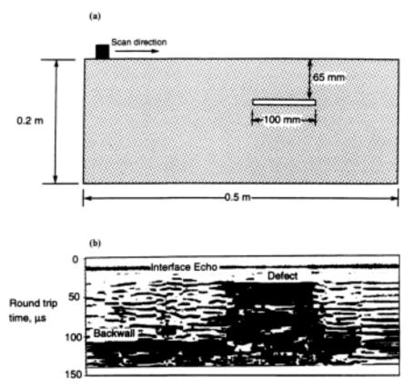
**Figure 8.8** Imagining of defect in concrete using ultrasonic pulse-echo technique, (a) Cross section of test specimen; (b) B-scan. Based on ref. 55.
