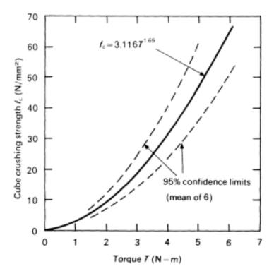
Figure 4.19 Typical compressive strength/torque calibration (based on ref. 96).
