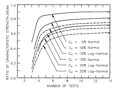
**Figure 1.10** Characteristic strength (95% confidence limit) as a function of coefficient of variation and number of tests (based on ref. 13).
