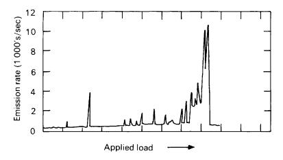
Figure 8.15 Typical acoustic emission plot (based on ref. 50).
