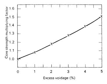
Figure 5.4 Excess voidage corrections (based on ref. 25).
