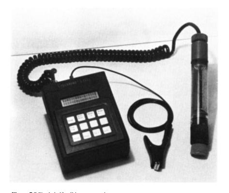
Figure 7.8 Single half-cell instrumentation.
