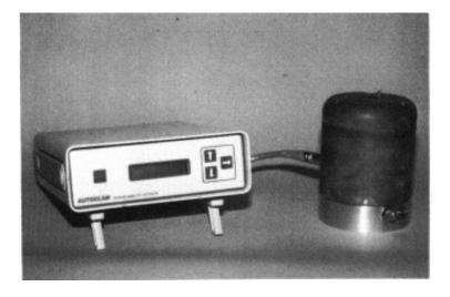
Figure 7.20 AUTOCLAM air and water permeability instrumentation.
