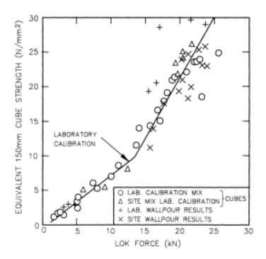
Figure 4.13 Low strength Lok-test correlation.
