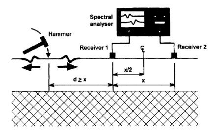
Figure 8.11 Spectral analysis of surface waves.
