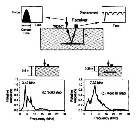
Figure 8.9 Frequency domain analysis of pulse-echo signal (based on ref. 265).
