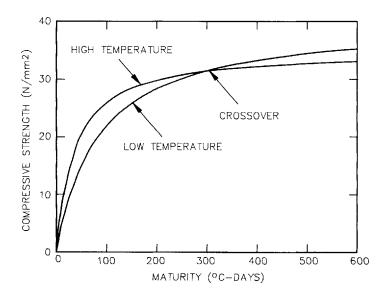
**Figure 8.19** The effect of early age curing temperature on the strength-maturity relationship (based on ref. 294).
