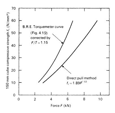
Figure 4.20 Comparison of calibration curves for natural aggregates (based on refs 96 and 97).
