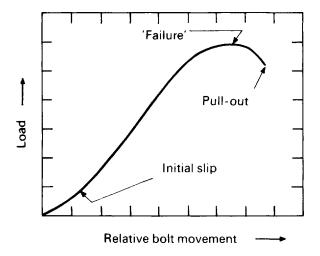
Figure 4.16 Typical loading curve.
