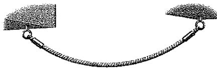
cables support their loads in tension (a)
