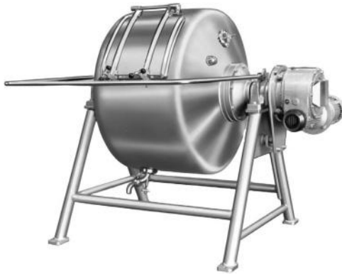
Figure 9.2. Batch butter churn (APV Unit Systems, Denmark). Fearon and Golding (2008).
