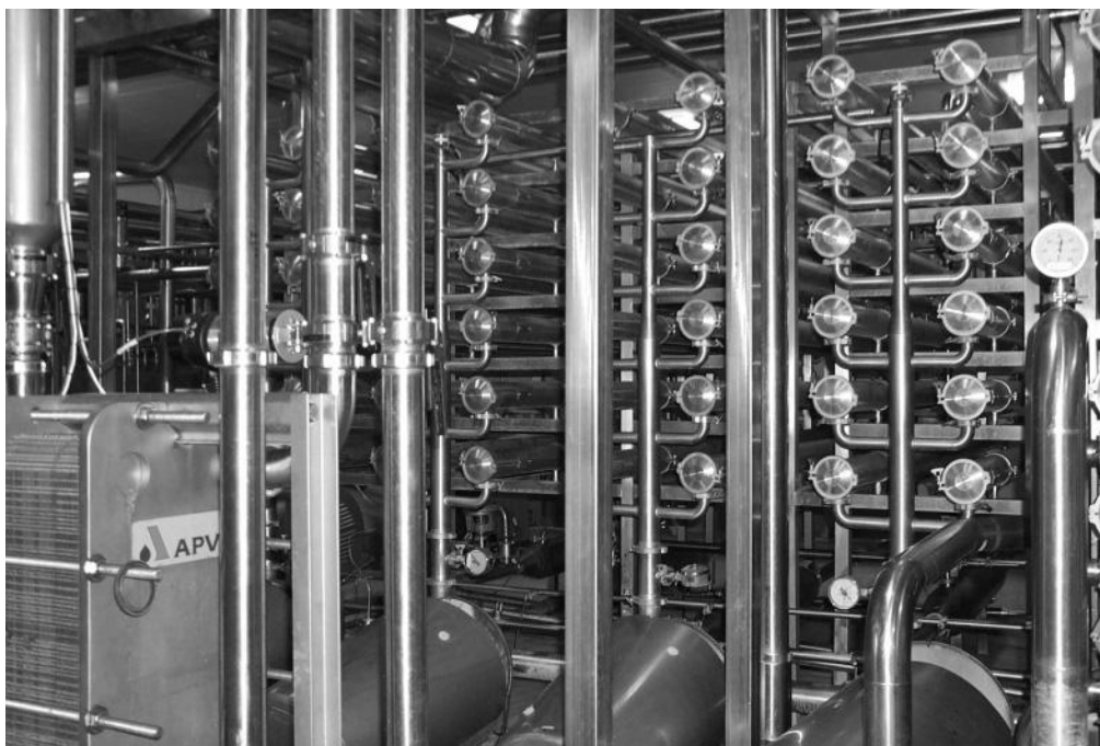
Figure 8.5. Spiral wound UF membrane unit. Reproduced by permission of Fonterra Co-operative Group Ltd.
