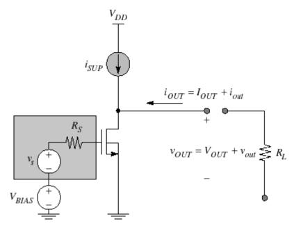
\* For DC bias analysis, the small-signal source (with  $R_S$ ) and the load resistor  $R_L$  are eliminated, along with the internal resistance  $r_{oc}$  of the current source
