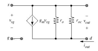
Transform this into a circuit with  $v_{gs}$  as the control voltage
