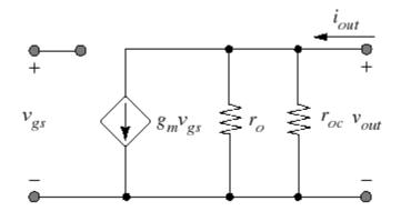
Tradeoffs are different from case of resistor load since  $I_D$  is now decoupled from the small-signal current supply resistance  $r_{oc}$
