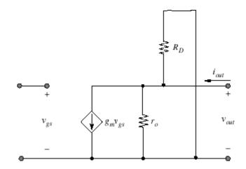
Find two-port parameters of this amplifier:"natural" to use the transconductance form
