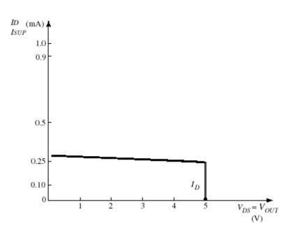
The region of input bias voltage  $V_{BIAS}$  for which the current source and the MOSFET are in their constant-current regions is *extremely* small ....
