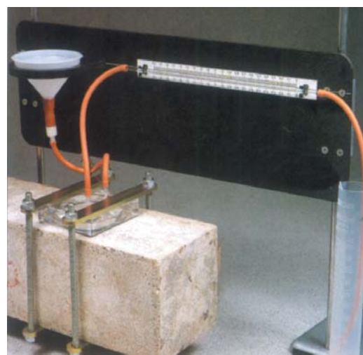
Cap and Initial Surface Absorption Test (ISAT)
