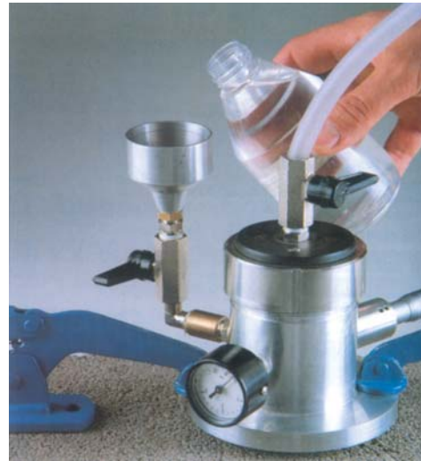
In-situ Water Permeability of Concrete
