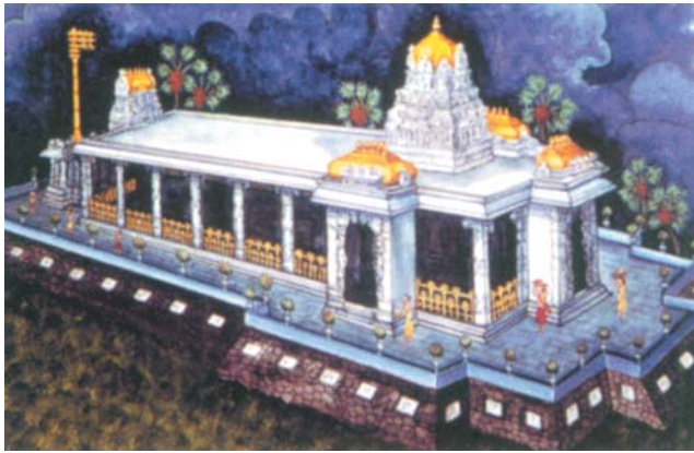
An architect's rendering of the Hindu Temple built at Kauai Island, Hawaii. A massive concrete foundation was laid to last for at least one thousand years. They have used high volume fly ash concrete replacing OPC by 57%.
