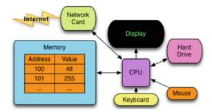
Fig. 2.1 Conceptual View of a Computer
