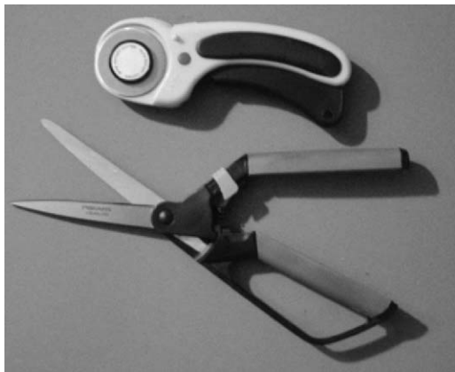
FIGURE 17-7 Examples of ergonomic cutting tools used in sewing and other crafts. Top , An ergonomic rotary cutter with an automatic closing safety feature. Bottom , Soft-handled scissors with a spring-loaded automatic opening feature.
