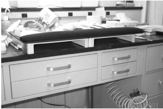
FIGURE 12-3 Ergonomic interventions need not be costly. Therapists can often find nontraditional applications for many items used on a daily basis and/or work aides. In this case, two monitor risers were placed side by side to provide 2 inches of height, atop which an old keyboard tray with a wrist rest was placed.
