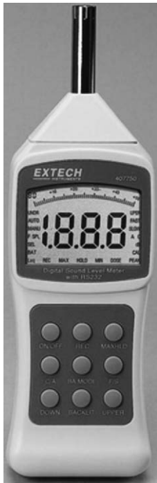
FIGURE 9-5 A sound level meter, used by ergonomists to measure noise. (Courtesy Exttech Instruments, Waltham, Mass.)
