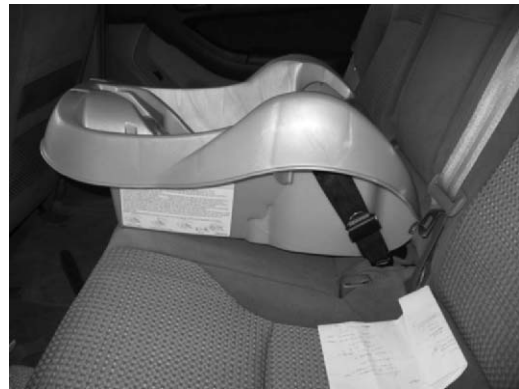
FIGURE A-3 Car seat coupling device.
