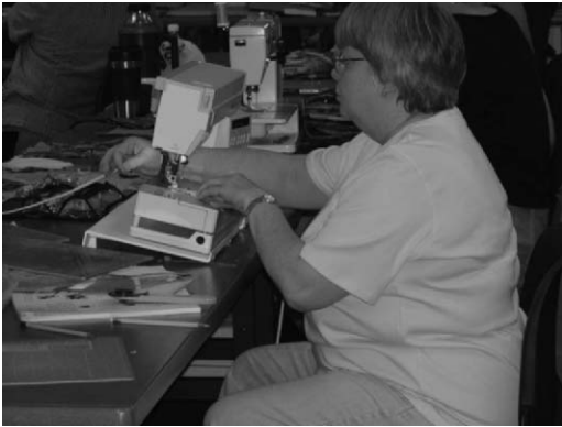
FIGURE 17-2 A wedge positioned under the sewing machine tilts the machine approximately 15 degrees and reduces neck and shoulder strain.
