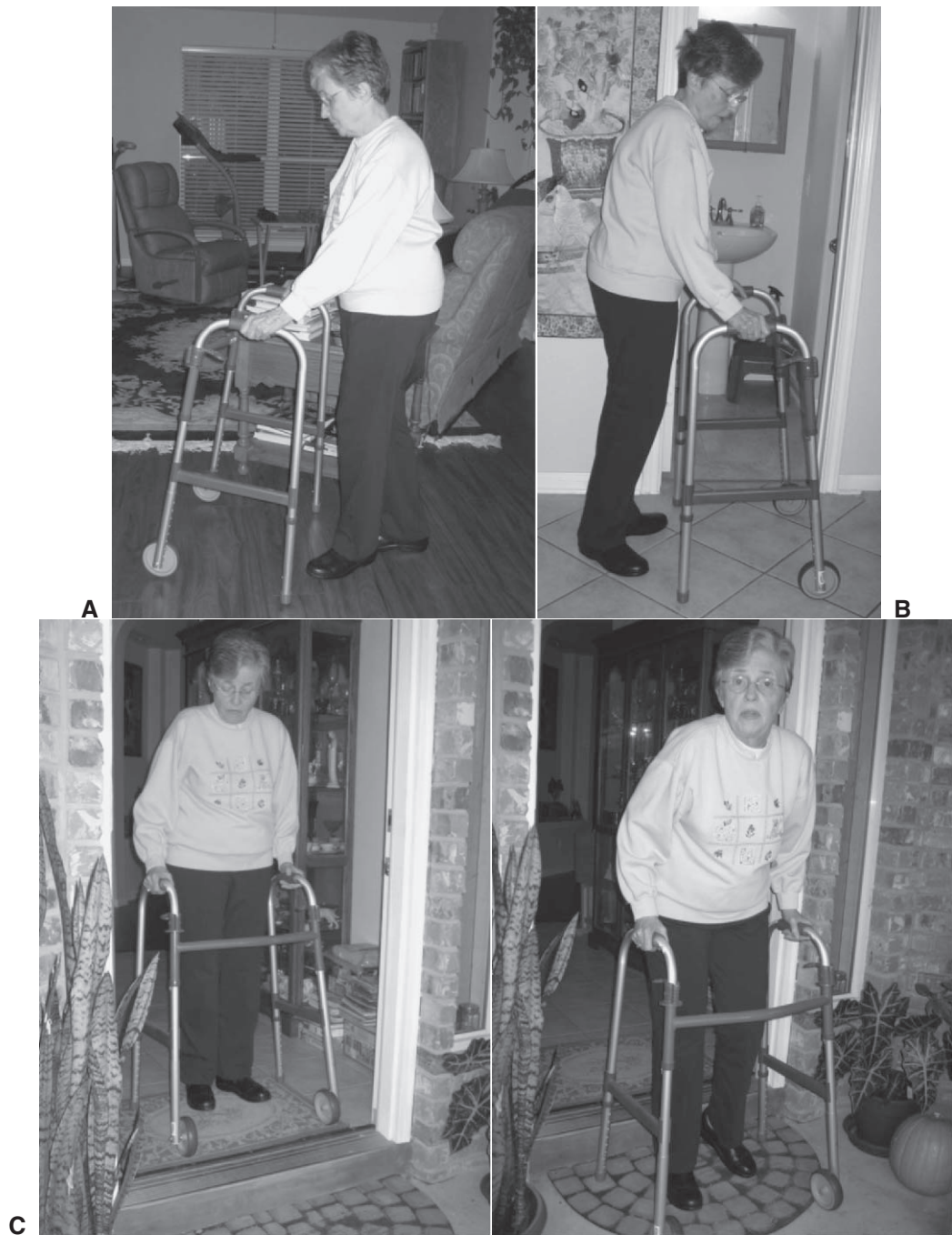
FIGURE 10-4 Evaluating the use of each walker in several tasks within the users' home environment allows the investigators to get accurate measures of ease-of-use, effectiveness, and efficiency. A , In this case, Mary Jo maneuvers around furniture and into her living room, where there is a large rug. B , She goes to the bathroom, but the walker does not fit through the doorway, so she must approach sideways and then hold onto the doorway itself. C and D , She exits her home down a single small step, which calls for balancing herself, lifting the walker, and placing it down the step—not an easy process!
