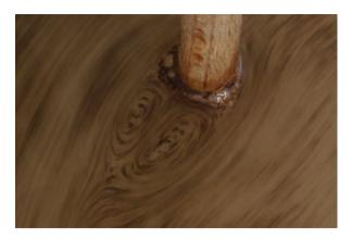
Fig. 4.7 A glimpse at unsteady recirculating vortices behind a cylinder at  $\text{Re}{\sim}330$  (photo of the author)
