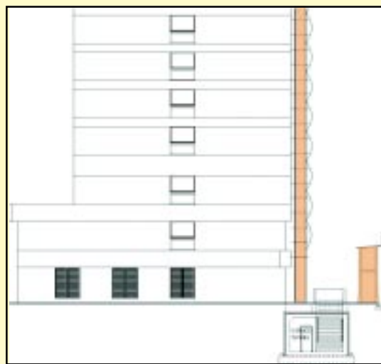
Figure 9 - Construction of double-layered scaffolding prior to renovation on facades
