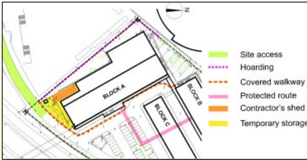
Figure 5 - Construction of New Rehabilitation Block
