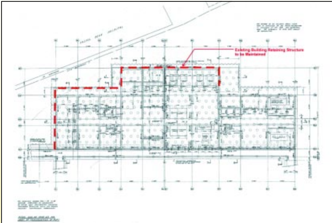
Figure 13 - Demolition of Block B - Existing Retaining Wall
