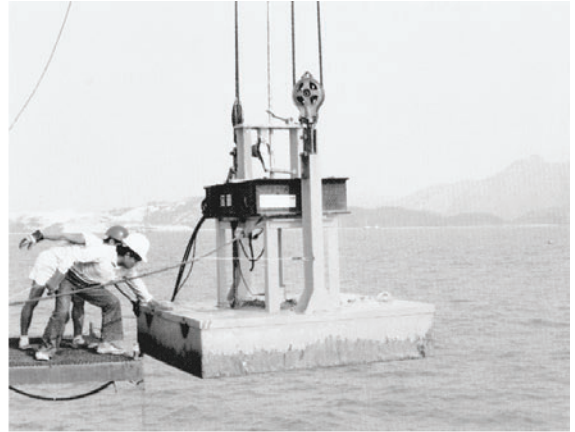
FIGURE 5.4 CPT sounding methods. (a) On land; (b) over water.
