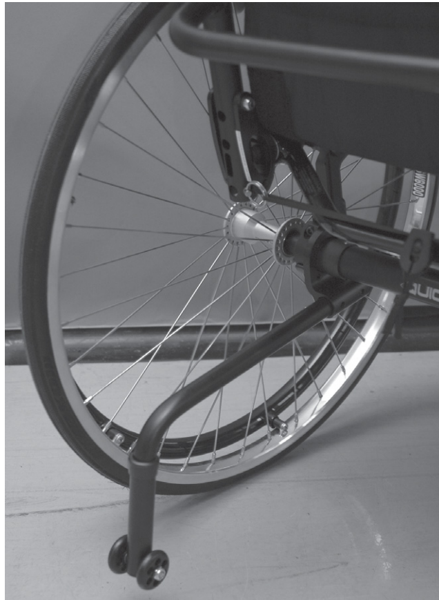
Figure 13.15 Anti-tip bars are attached to the back of wheelchairs to prevent them toppling over backwards.
