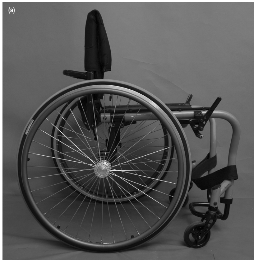
Figure 13.5 The back wheels can be placed low (a) or high (b) on the frame of the wheelchair. This changes the seat-to-floor distance, the rake of the seat and recline of the backrest. The vertical position of the back wheels determines how far above the seat the top of the wheels protrude. This has implications for transferring and for propulsion.
