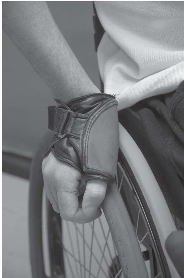
Figure 13.11 Textured gloves used in conjunction with a rubberized pushrim help patients with limited hand function push. The tyre is solid.
