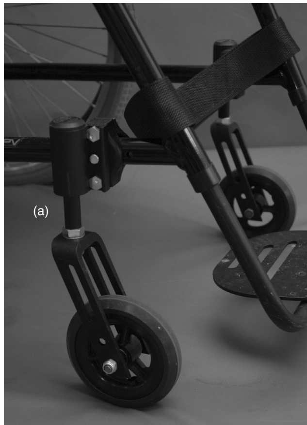
Figure 13.10 The stems of the castors (a) need to be perpendicular to the floor, otherwise they vibrate and the wheelchair is more difficult to push.
