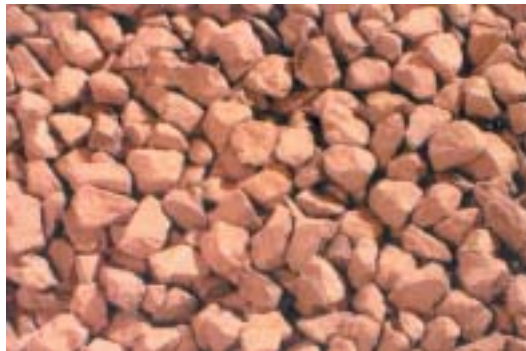
Barmac crushed 20 mm cubical aggregate. It will make good concrete.
