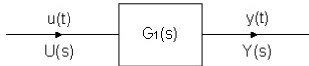
Figure 2.3 Block representation of a transfer function
