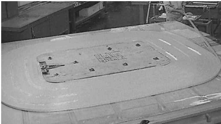
FIGURE 2.1.12 Pancake winding during winding process.
