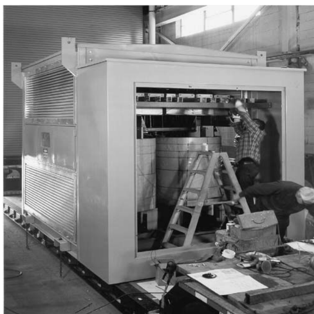
FIGURE 2.4.20 A 24-pulse dry-type transformer. 7000-kVA drive duty transformer, to be located in a tunnel, made of two 3500-kVA 12-pulse transformers. Each core and coil has 1100-V delta and wye secondary windings. Each core and coil has a 13,200-V extended-delta primary winding. One core and coil has its primary winding shifted -15^\circ , while the other core and coil has its primary winding shifted +15^\circ . One reconnectable primary spare core and coil can be used to replace either core and coil assembly. (Photo courtesy of Niagara Transformer Corp.)
