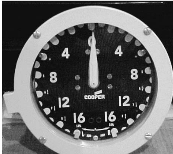
FIGURE 2.7.15 Tap-changer position indicator.
