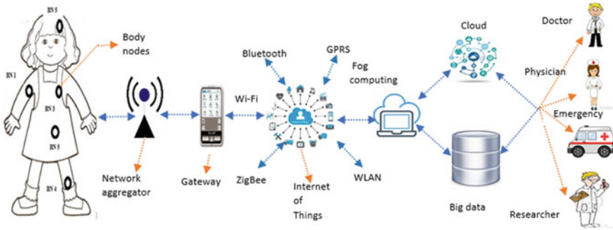
Fig. 1 Overall architecture diagram of WBAN
