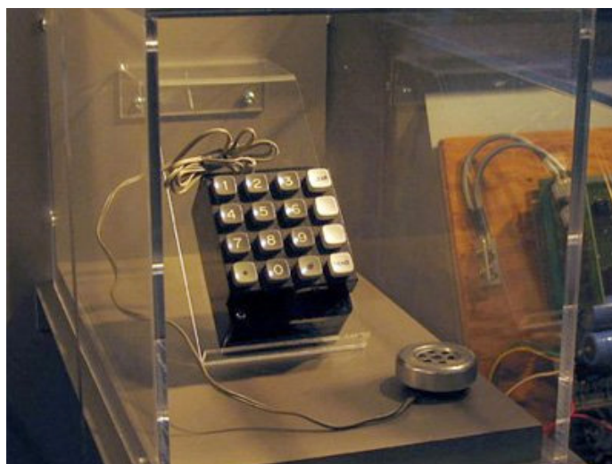
Figure 2.1: The blue box built by Steve Wozniak, on display at the Computer History Museum
