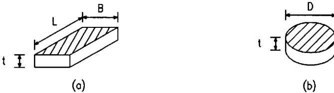
Fig. 28.2 Elastomeric bearing dimensions for (a) a rectangular block, (b) a circular block
