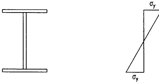
Fig. 17.11 Design stresses for non-compact sections
