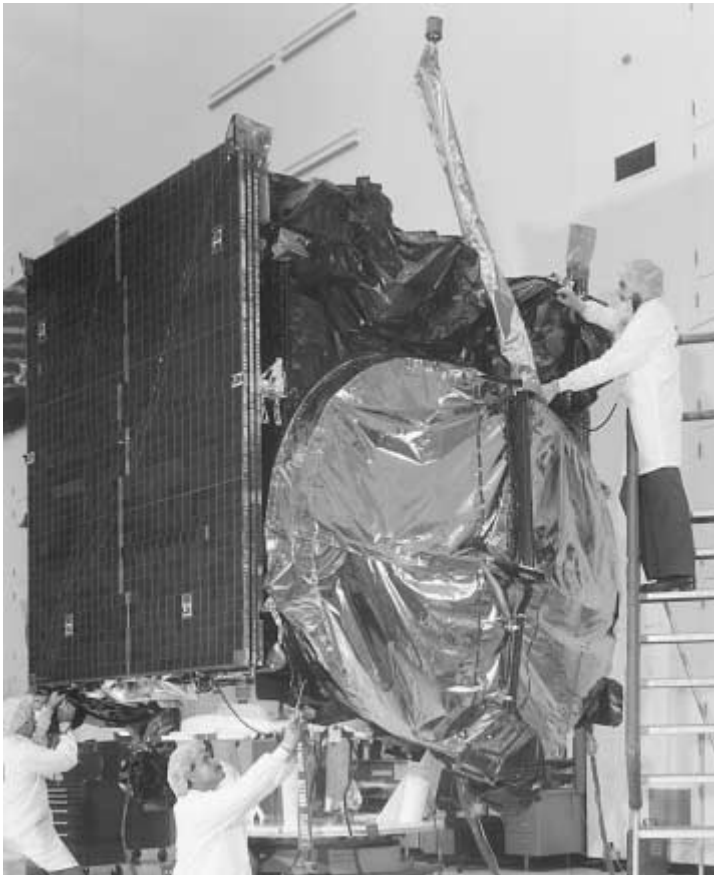
Figure 7.2 Aussat B1 (renamed Optus B), Hughes first HS 601 communications satellite is prepared for environmental testing. (Courtesy of Hughes Aircraft Company Space and Communications Group.)
