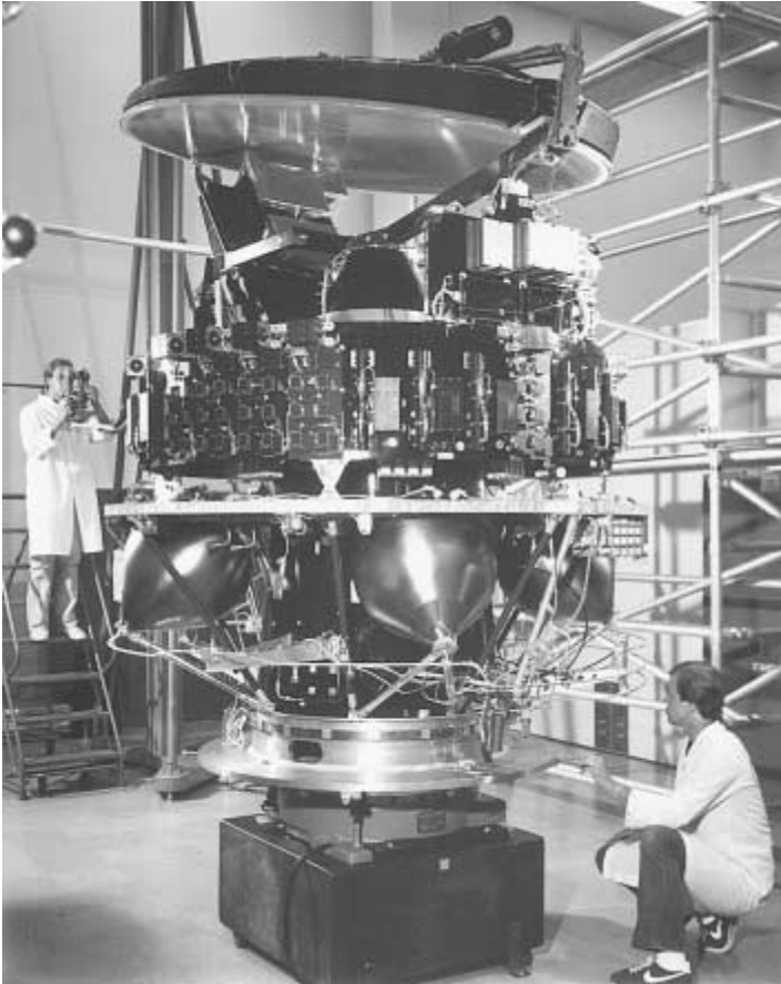
Figure 7.7 Technicians check the alignment of the Telestar 3 communications satellite, shown without its cylindrical panels. The satellite, built for the American Telephone and Telegraph Co., carries both traveling-wave tube and solid-state power amplifiers, as shown on the communications shelf surrounding the center of the spacecraft. The traveling-wave tubes are the cylindrical instruments. (Courtesy of Hughes Aircraft Company Space and Communications Group.)
